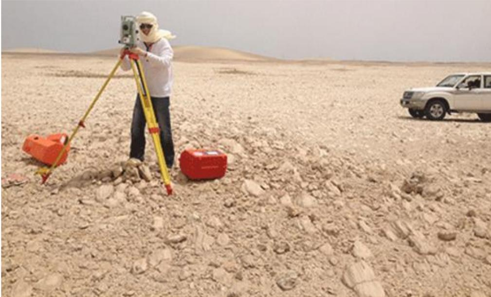
**Figure 5.** Leica builder 300 theodolite
