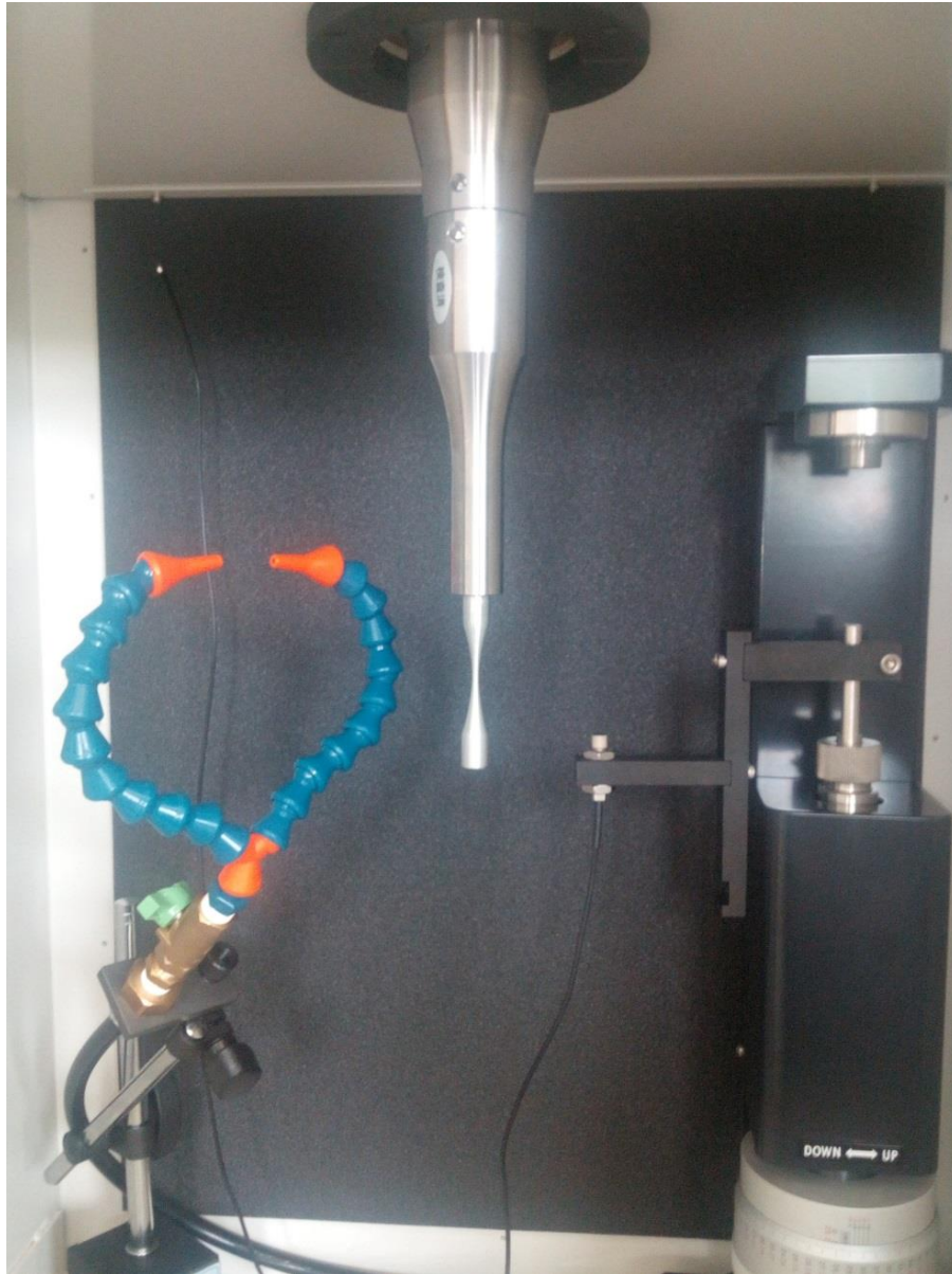
Fig. 2. Aluminum specimen sample screwed to the horn of SHIMADZU ultrasonic fatigue testing machine (USF-2000)
