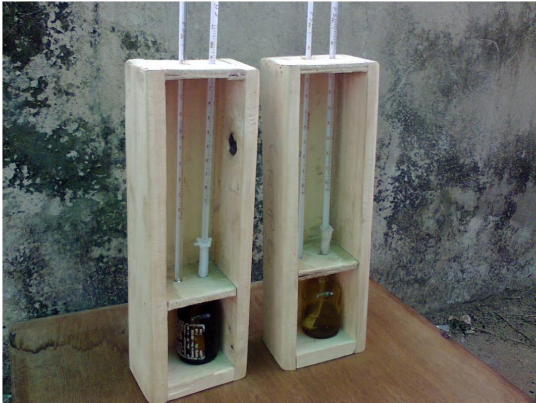
Figure 5. Locally constructed Hygrometer
