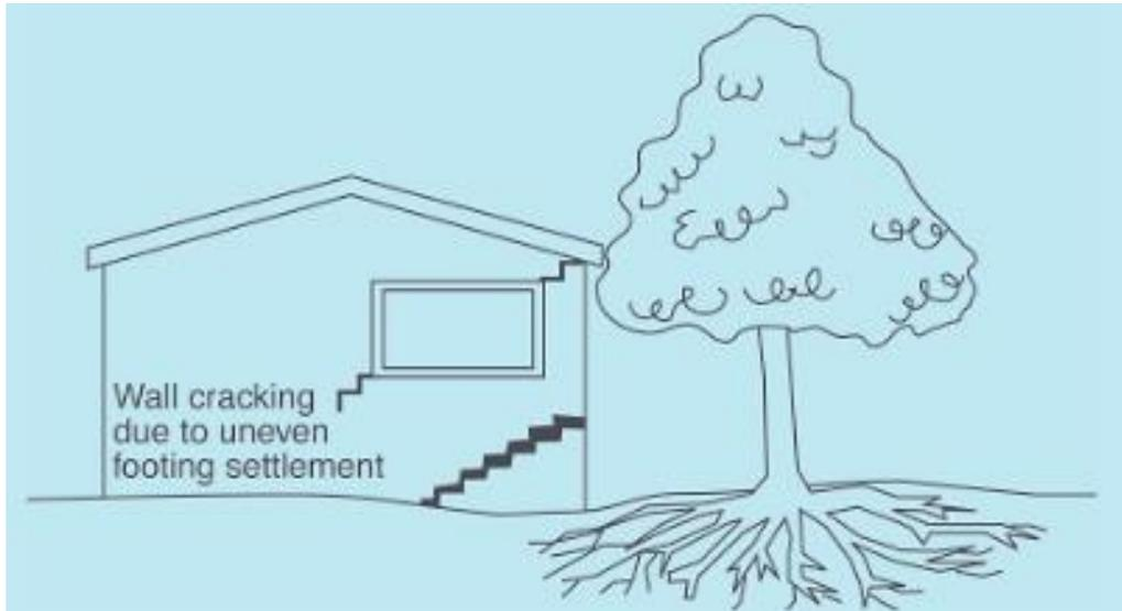
**Figure 5.** Trees can cause shrinkage and damage
