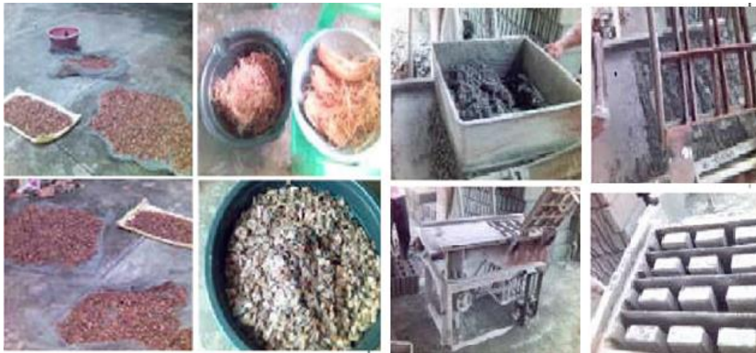
Figure 6. Preparation and Molding of CHB with coconut shell and fiber
