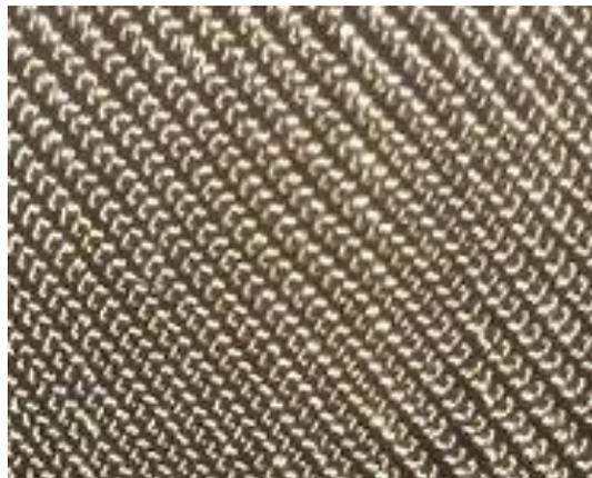
**Figure 1.** Basalt fabric with twill weaves
