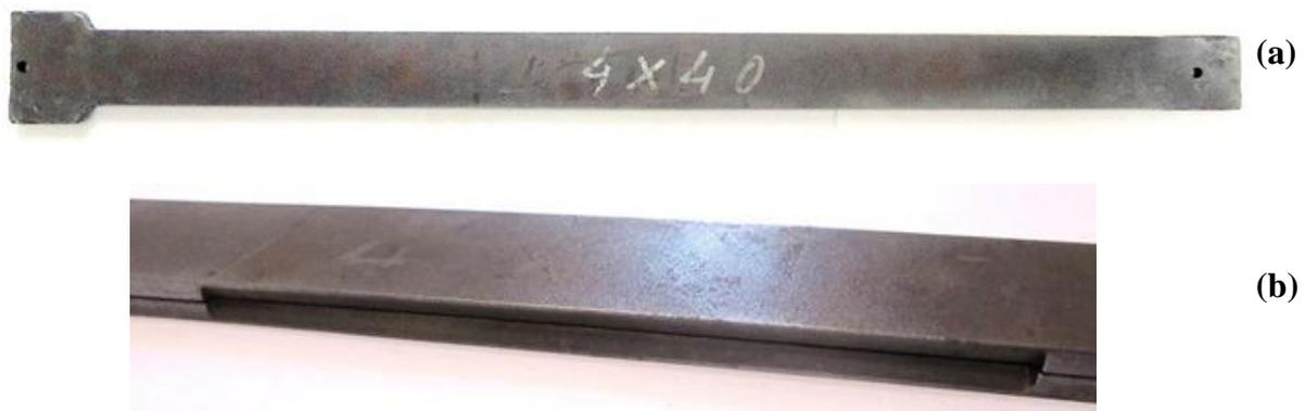
**Figure 3.** The test kit before hardening process.
