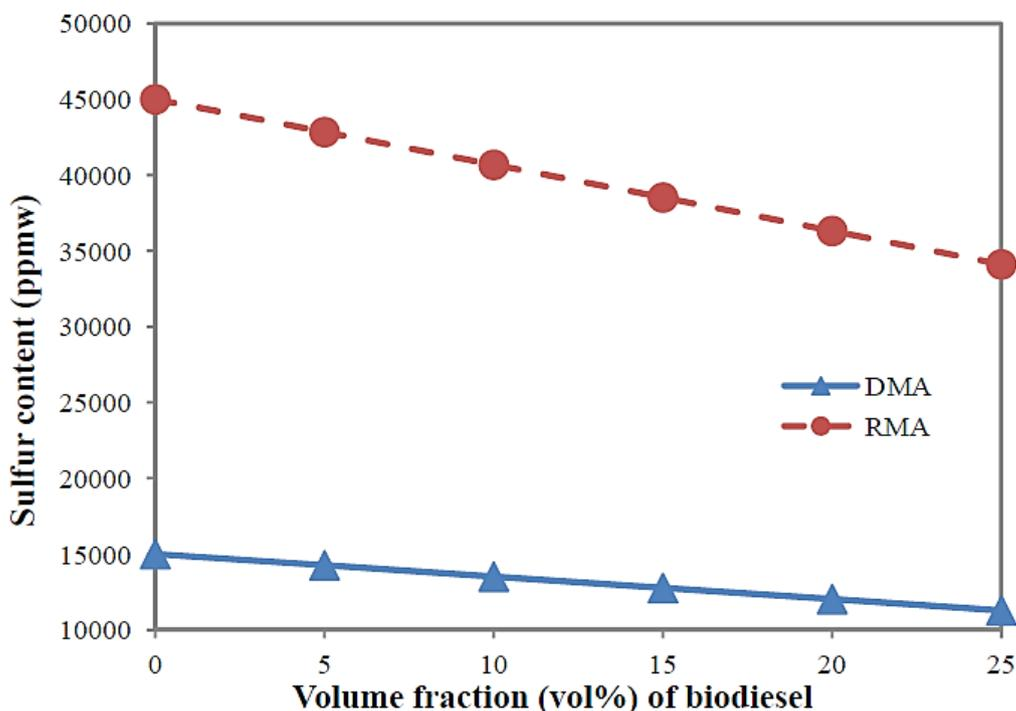
**Figure 6.** Variation of sulfur content with volume fraction of biodiesel blends in distillate marine fuel DMA and residual marine fuel RMA.
