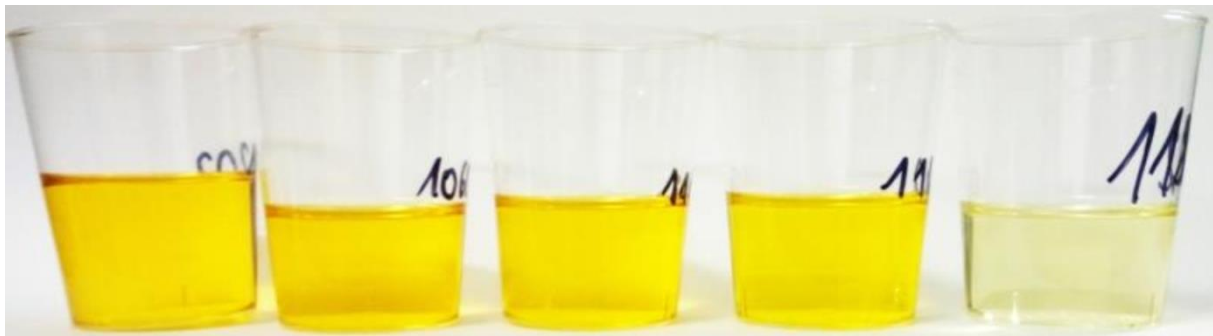
Figure 3. Photo showing the color change of samples of refined olive oil depending on the temperature of their incubation (from the left: 20 °C, 60 °C, 100 °C, 140 °C and 180 °C)
