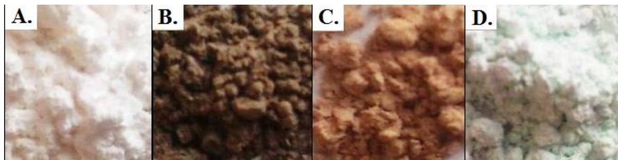
**Figure 3.** Photos of obtained powders: A.  $\text{KTaO}_3$ , B.  $\text{KTa}_{0.8}\text{Co}_{0.2}\text{O}_3$ , C.  $\text{KTa}_{0.8}\text{Fe}_{0.2}\text{O}_3$ , D.  $\text{KTa}_{0.8}\text{Ni}_{0.2}\text{O}_3$
