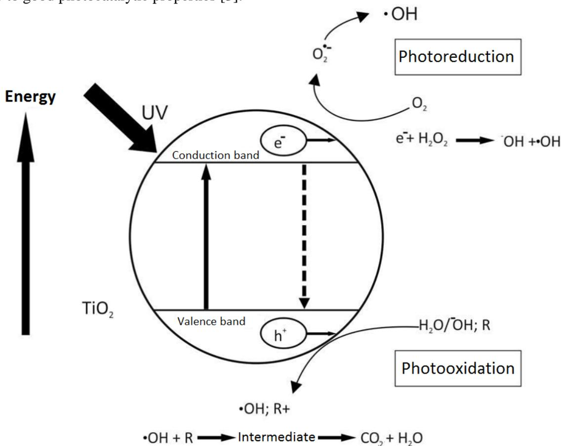
**Figure 1.** Scheme of photocatalysis on the  $\text{TiO}_2$
