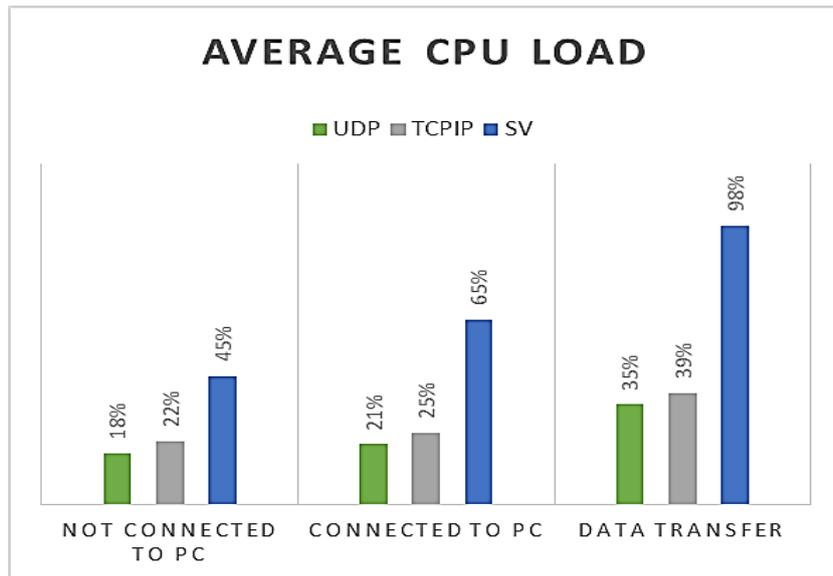
**Figure 6.** Average CPU load with different data protocols and states of robot
