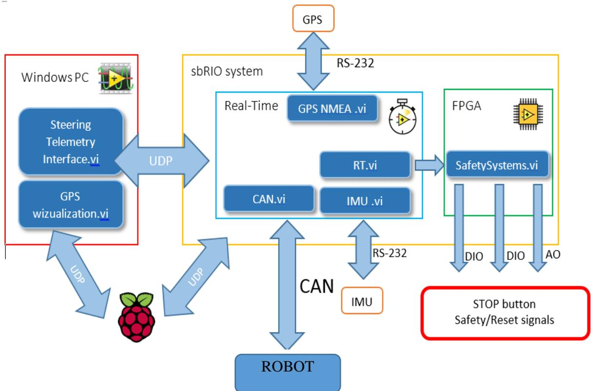
**Figure 2.** Control architecture
