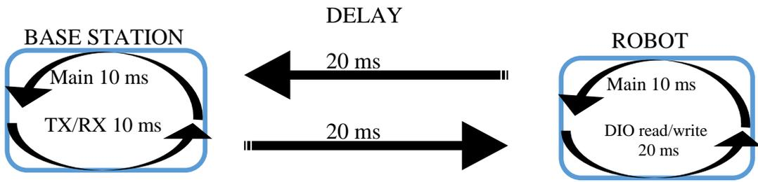
**Figure 4.** Timing structure of system
