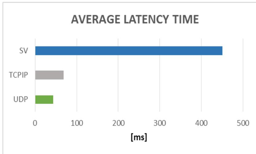
**Figure 5.** Average delay for different data protocols.
