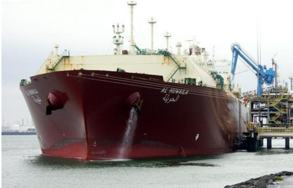
**Figure 2.** LNG tanker, Q-flex type, Al Huwaila.
