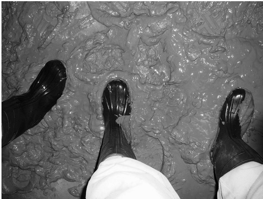
Figure 6. Fly ash – saline water slurry two weeks after placement in an underground working during liquidation works. The slurry is still liquid but able to withstand a pressure of no less than about 20 kPa
