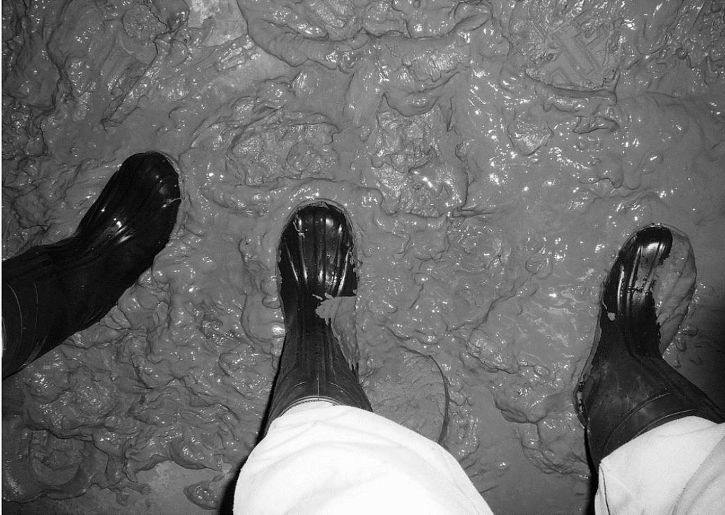
**Figure 6.** Fly ash – saline water slurry two weeks after placement in an underground working during liquidation works. The slurry is still liquid but able to withstand a pressure of no less than about 20 kPa.
