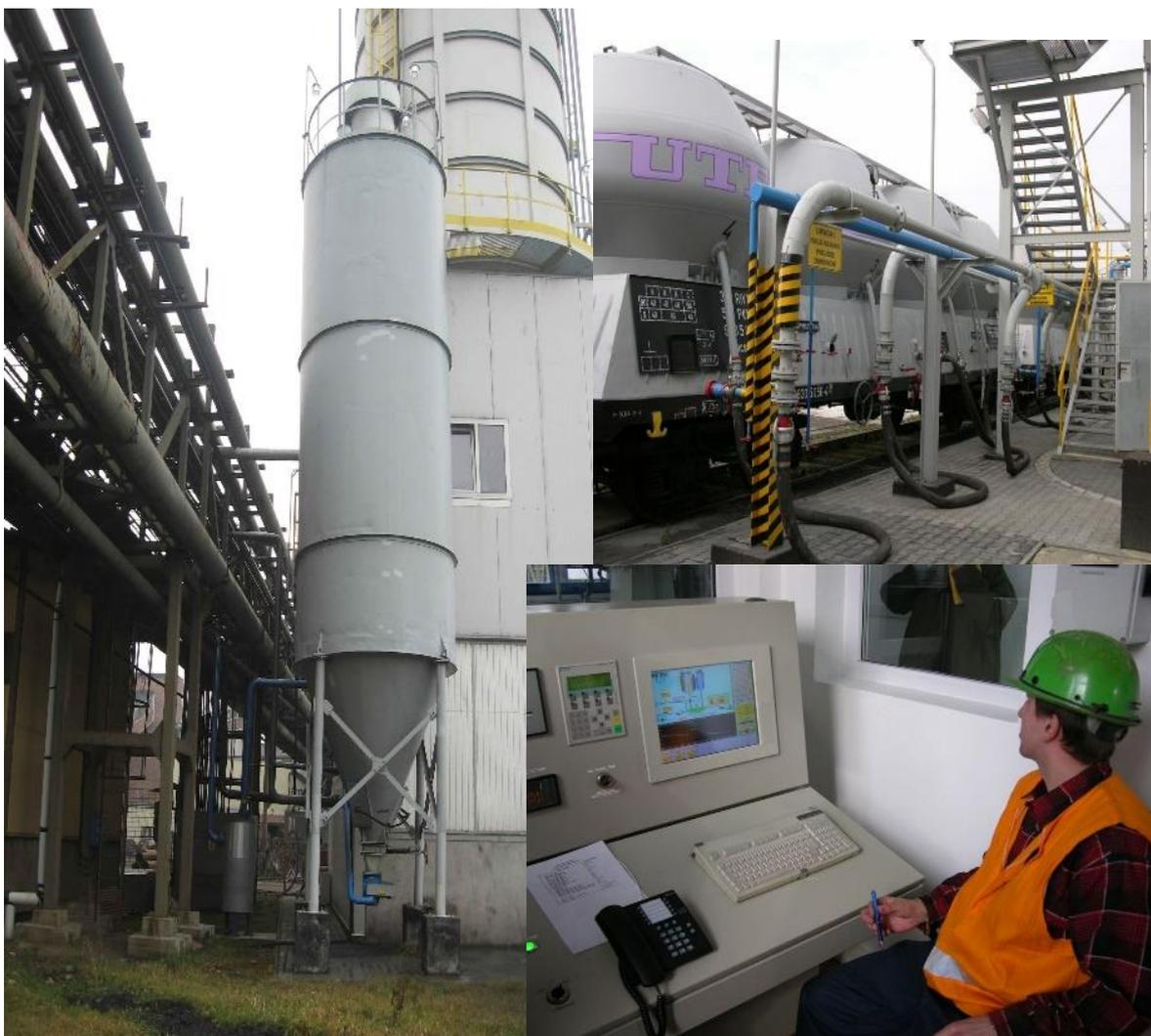
**Figure 3.** Fly ash – water slurry preparation plan at “Szczygłowie” mine. On the left: fly ash tank and main building behind binder tank, right up: pneumatic fly ash discharge from tank wagon. Right down: control room (Palarski et. al., 2011).
