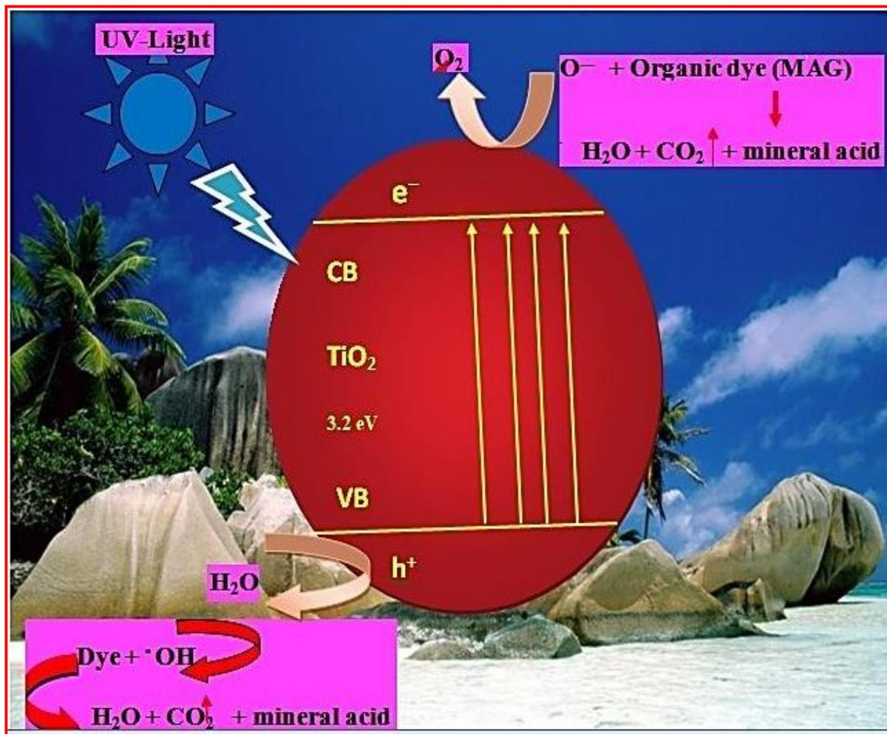
**Scheme 2.** Schematic diagram of photodegradation of MAG on TiO<sub>2</sub> nanomaterial under UV-light for successive mineralization.
