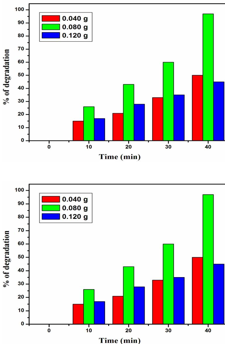
**Fig. 7.** Different catalyst loading upon MAG dye under UV-light irradiation by TiO<sub>2</sub> nanomaterial is degradation of MAG dye
