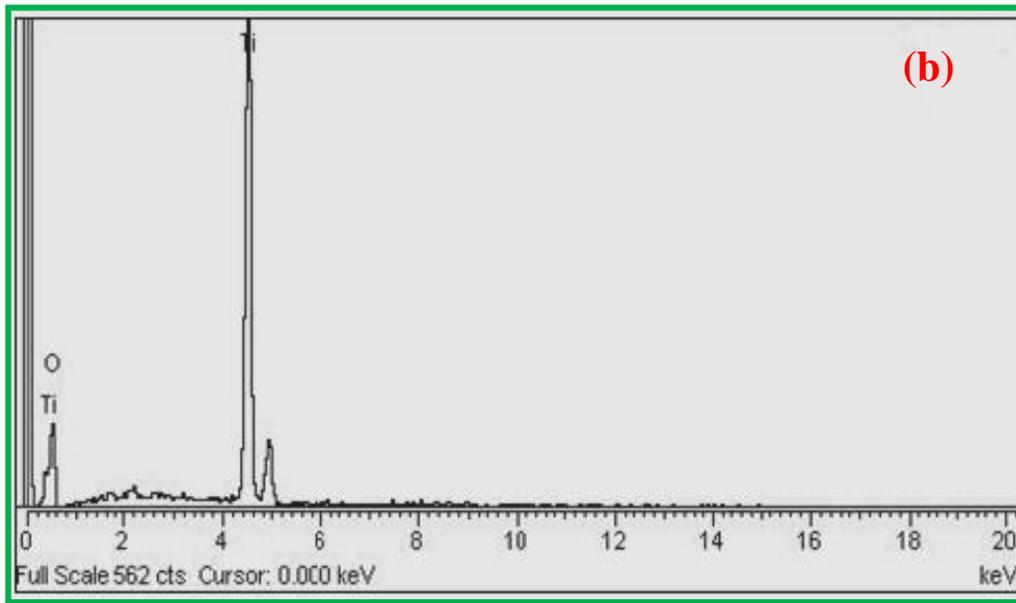
**Fig. 2.** HR-SEM image of (a) TiO<sub>2</sub> (b) EDX analysis of TiO<sub>2</sub> nanocomposite material
