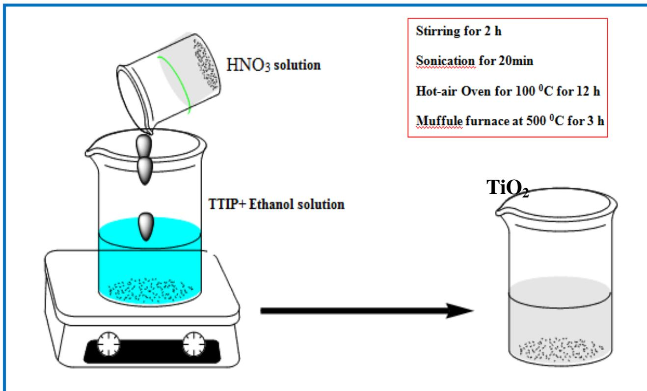
**Scheme 1.** Schematic representation for preparation of TiO<sub>2</sub> nanomaterial
