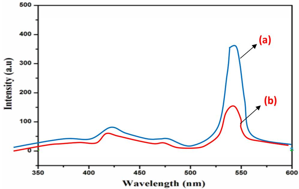
Fig. 5. PL spectra of (a) TiO<sub>2</sub> and (b) TiO<sub>2</sub> P25 nanomaterial
