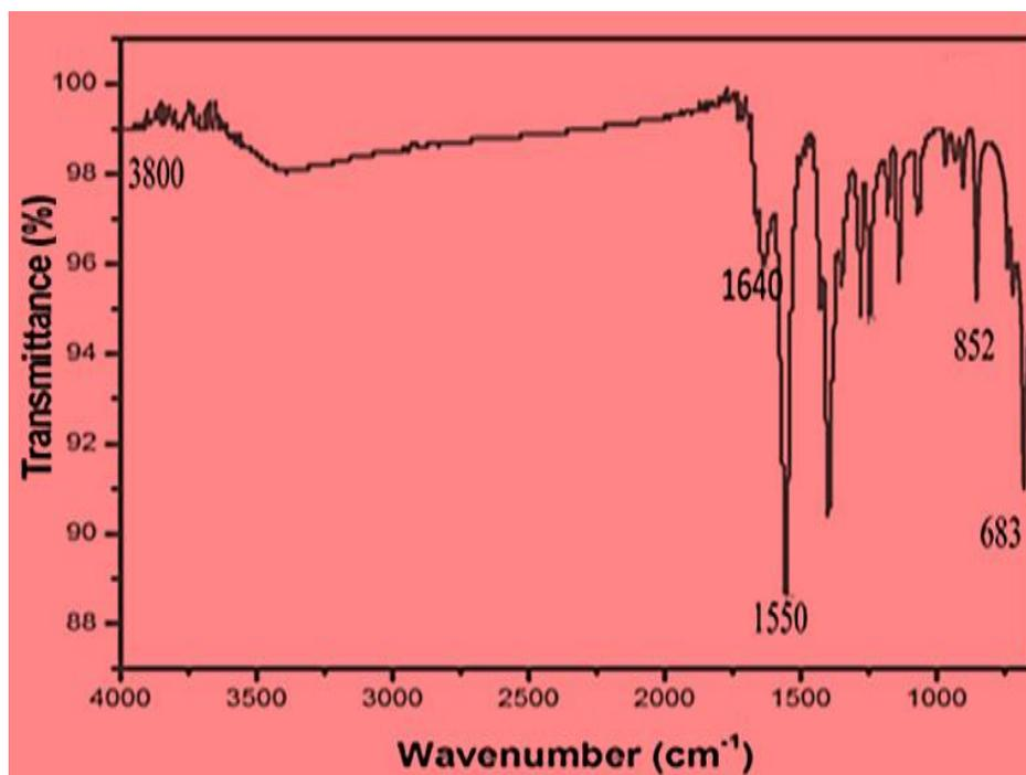
Fig. 4. FT-IR spectra of TiO<sub>2</sub> nanomaterial
