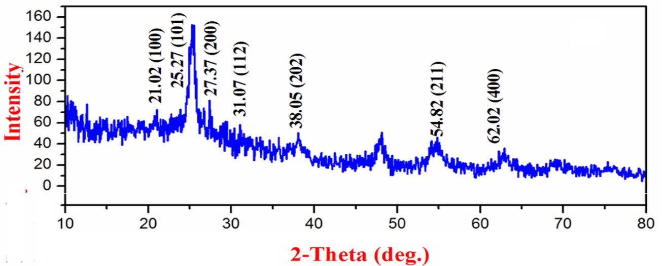
**Fig. 3.** XRD analysis of TiO<sub>2</sub> nanocomposite material
