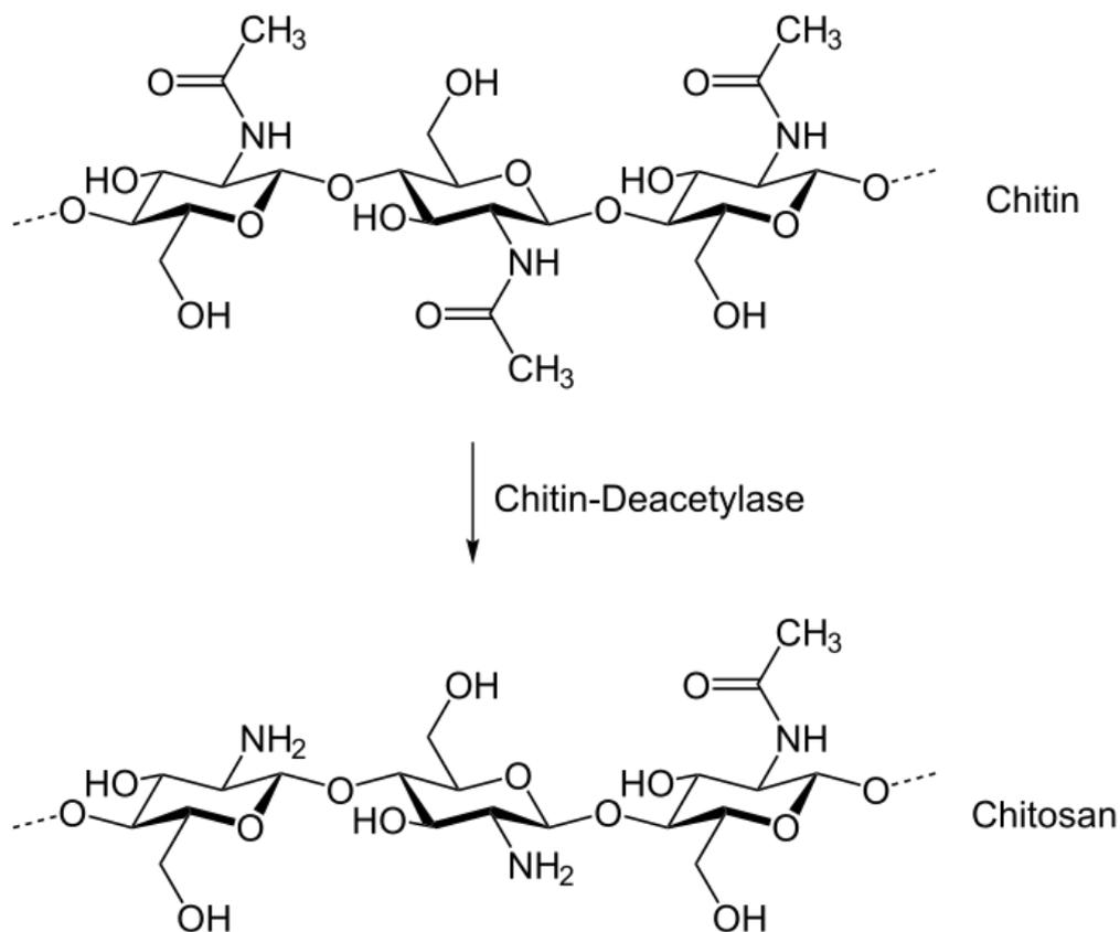
**Figure 1.** Synthesis of chitosan
