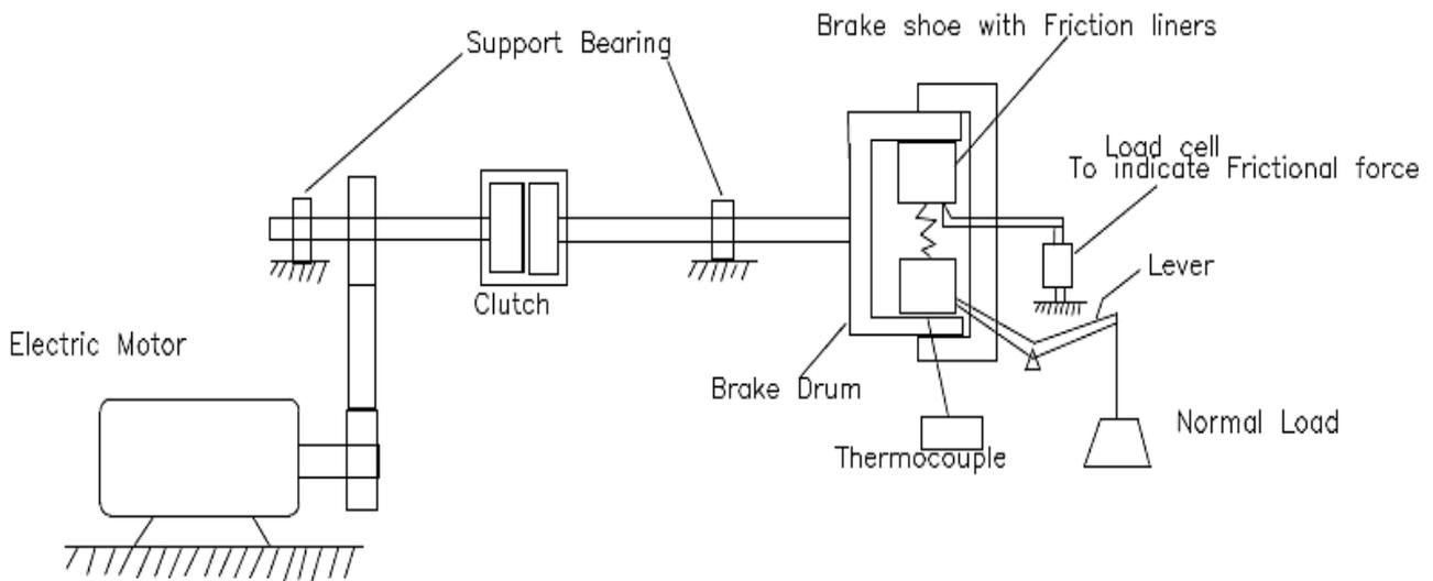
**Figure 1.** Proposed test set up.
