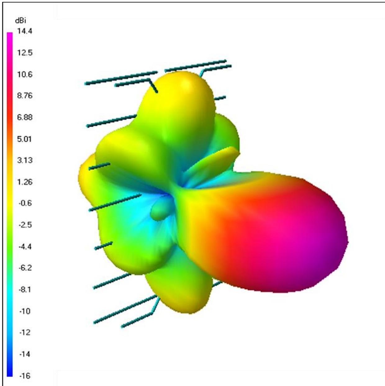
**Figure 2.** Radiation pattern in 3D at 700 MHz
