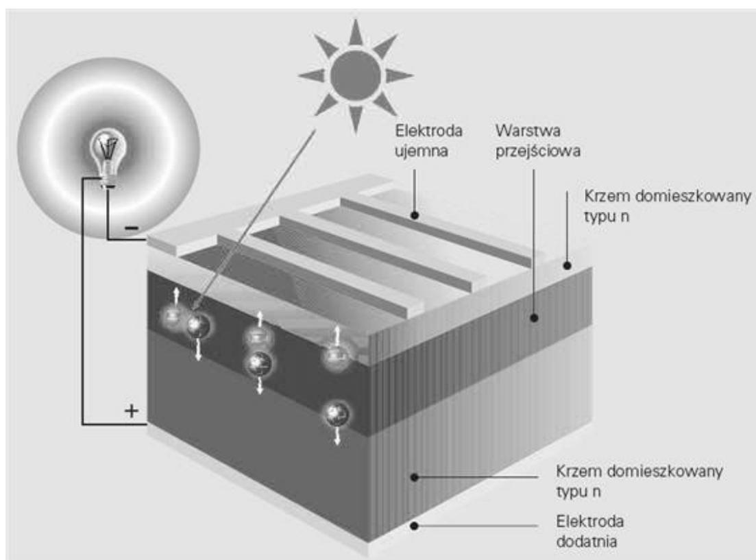
**Fig. 1.** Operation principle of a photovoltaic installation
