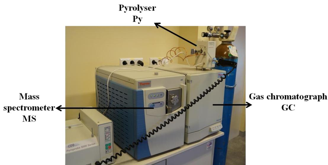
**Figure 3.** Measuring station for chromatographic analysis (Py-GC/MS method).
