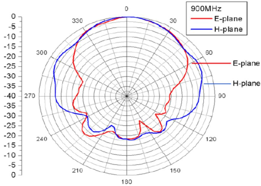
Figure 7. The variation of E field pattern, H-field pattern, vertical azimuth pattern and horizontal azimuth pattern at 900 MHz
