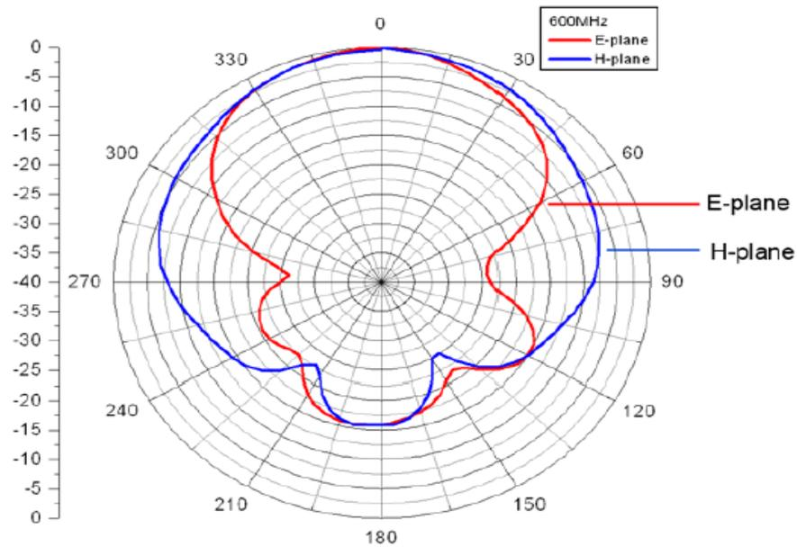
Figure 4. The variation of E field pattern, H-field pattern, vertical azimuth pattern and horizontal azimuth pattern at 600 MHz
