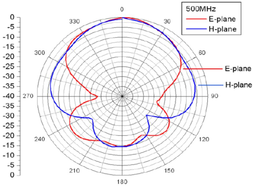
Figure 3. The variation of E field pattern, H-field pattern, vertical azimuth pattern and horizontal azimuth pattern at 500 MHz
