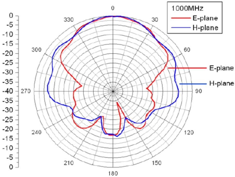
Figure 8. The variation of E field pattern, H-field pattern, vertical azimuth pattern and horizontal azimuth pattern at 1000 MHz
