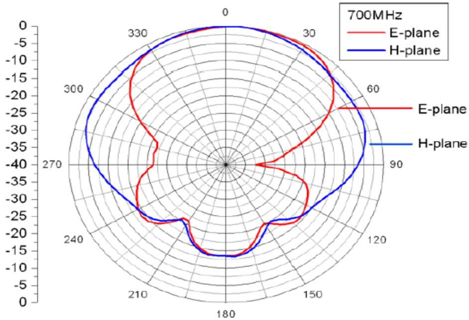
Figure 5. The variation of E field pattern, H-field pattern, vertical azimuth pattern and horizontal azimuth pattern at 700 MHz
