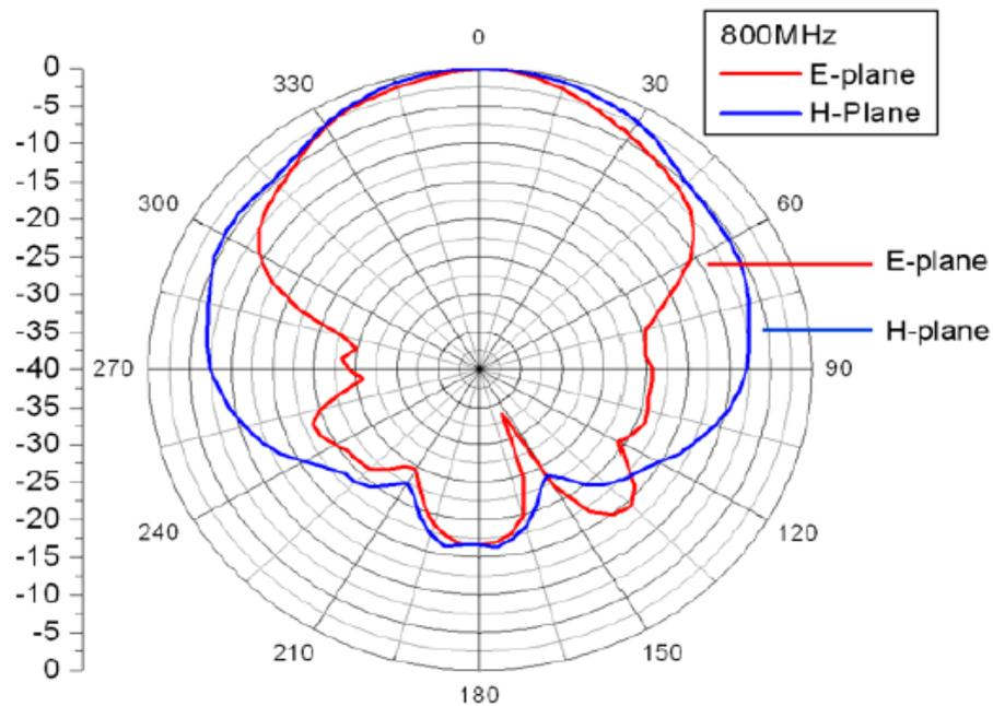
Figure 6. The variation of E field pattern, H-field pattern, vertical azimuth pattern and horizontal azimuth pattern at 800 MHz
