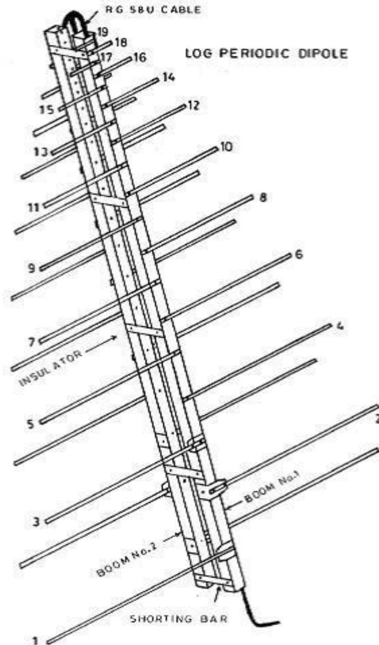
**Figure 1.** The schematic diagram of LPDA.
