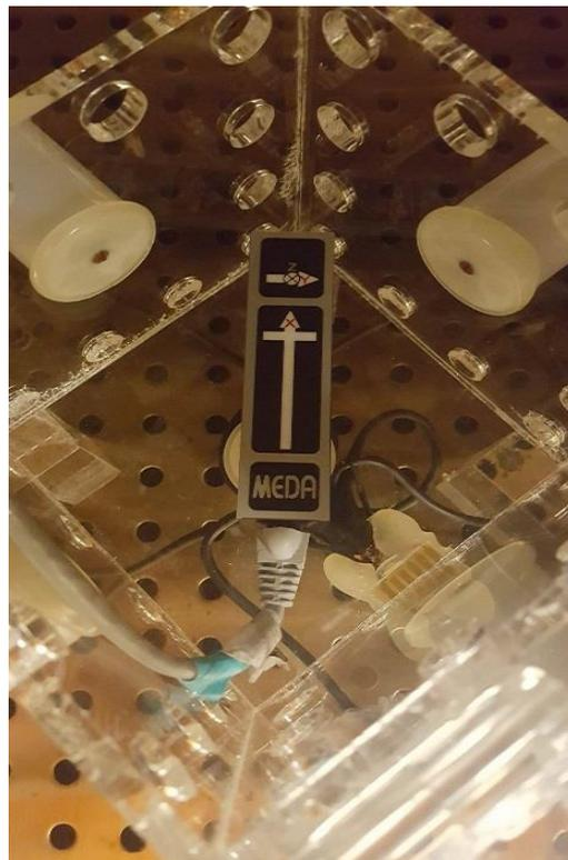
**Figure 2.** The FVM-400 sensor positioned within the 4D box within the incubator.
