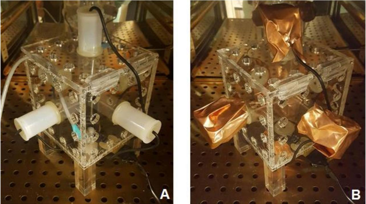
**Figure 1.** The 4D box within the incubator without (A) and with (B) copper-shielding surrounding the external surfaces of the solenoids.
