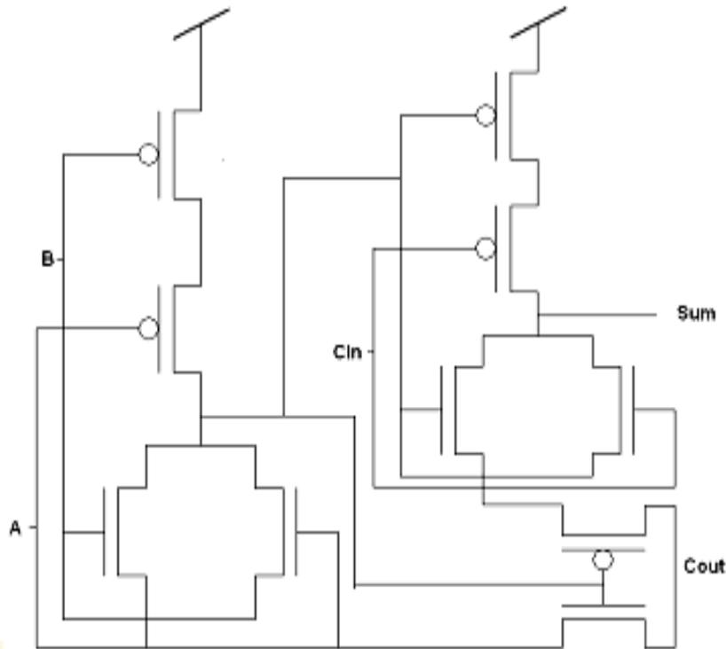
**Fig. 3.** SERF adder circuit with 10T
