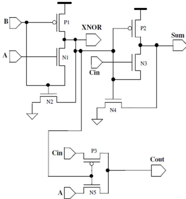
**Fig. 12.** Full adder using two XNOR gates and multiplexer
