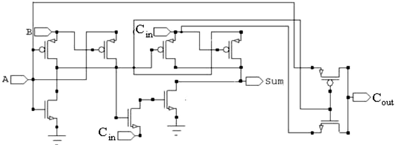
Fig. 11. 9T Full adder with extra added nMOS [ 14]
