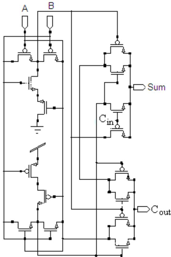
Fig. 5. 16T full adder using Transmission gates.
