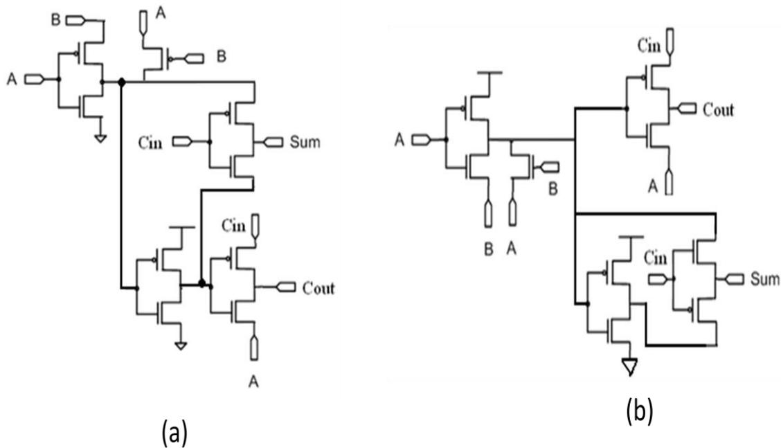
**Fig. 10.** 9T Full adders using XOR and XNOR cells
