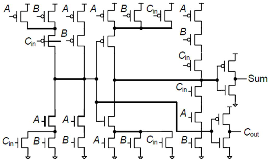
Fig. 1 – conventional 28T full adder circuit.
