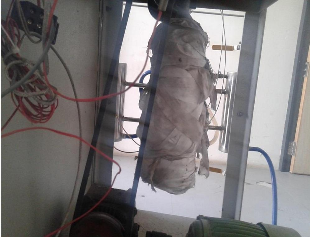
**Figure 4.** Char Tank to collect solid biofuel (5.84 liters capacity).
