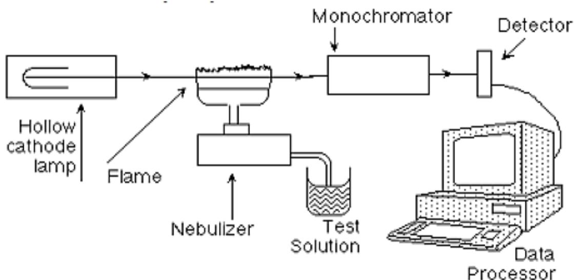
**Fig. 7.** Experimental design of Atomic Absorption Spectrophotometer.
