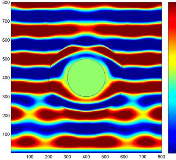
**Figure 6.** Electric field intensity distribution in z direction for electromagnetic slab or magnitude of pressure distribution for acoustic slab of  $R_1 = 0.1\text{m}$  and  $R_2 = 0.2\text{m}$  at 1800 time step. Black lines indicate inner and outer surfaces.
