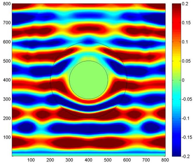
**Figure 5.** Electric field intensity distribution in z direction for electromagnetic slab or magnitude of pressure distribution for acoustic slab of  $R_1 = 0.1\text{m}$  and  $R_2 = 0.2\text{m}$  at 1400 time step. Black lines indicate inner and outer surfaces.
