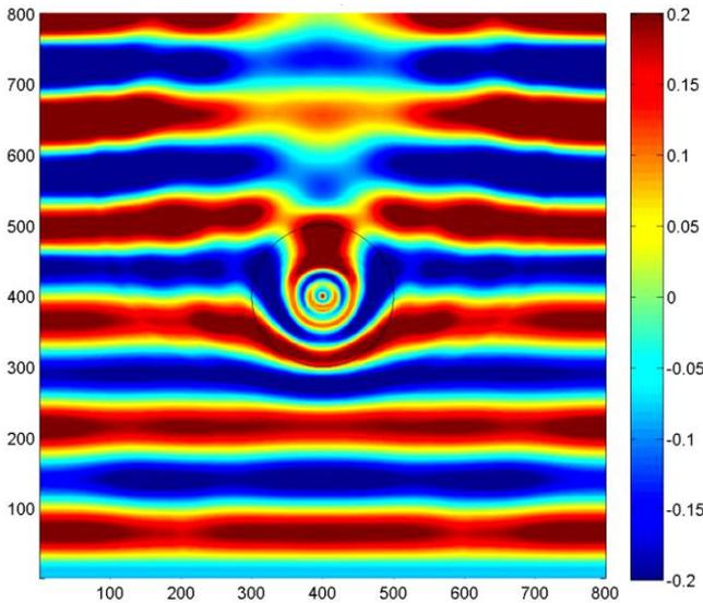
**Figure 8.** Electric field intensity distribution in z direction for electromagnetic slab or magnitude of pressure distribution for acoustic slab of  $R_1 = 0.1$  m and  $R_2 = 0.2$  m at 1600 time step. Black lines indicate inner and outer surfaces.
