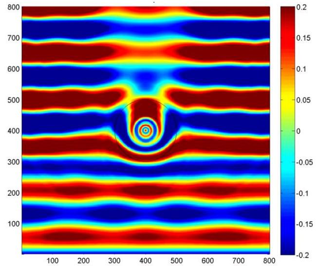
**Figure 9.** Electric field intensity distribution in z direction for electromagnetic slab or magnitude of pressure distribution for acoustic slab of  $R_1 = 0.1$  m and  $R_2 = 0.2$  m at 1800 time step. Black lines indicate inner and outer surfaces.
