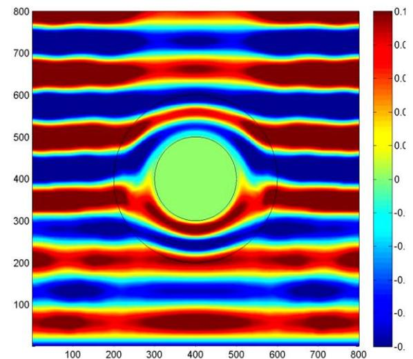
**Figure 4.** Electric field intensity distribution in z direction for electromagnetic slab or magnitude of pressure distribution for acoustic slab at 1800 time step. Black lines indicate inner and outer surfaces.
