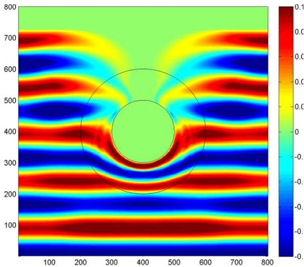
**Figure 3.** Electric field intensity distribution in z direction for electromagnetic slab or magnitude of pressure distribution for acoustic slab at 1000 time step. Black lines indicate inner and outer surfaces.
