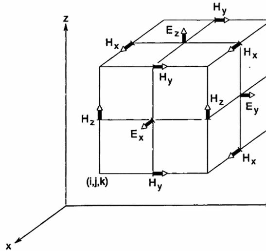
**Figure 1.** Positions of the electric and magnetic field components about a cubic unit cell of the Yee space lattice [5]
