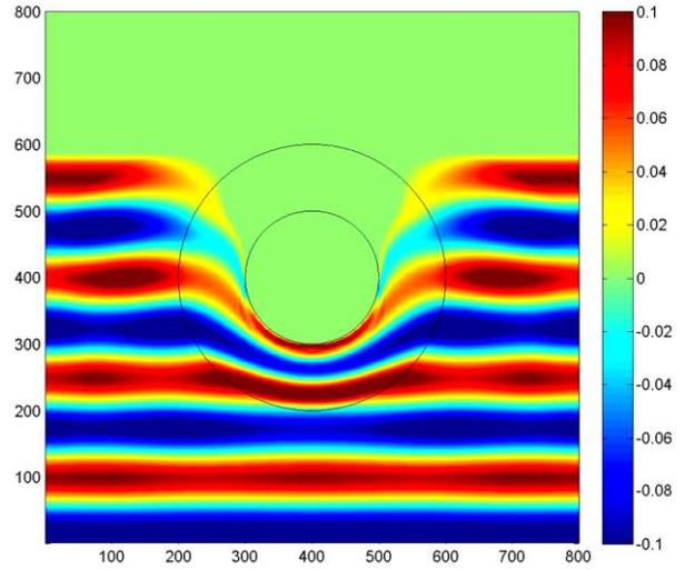
**Figure 2.** Electric field intensity distribution in z direction for electromagnetic slab or magnitude of pressure distribution for acoustic slab at 800 time step. Black lines indicate inner and outer surfaces.
