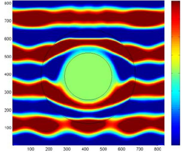
**Figure 7.** Electric field intensity distribution in z direction for electromagnetic slab or magnitude of pressure distribution for acoustic slab of  $R_1 = 0.125\text{m}$  and  $R_2 = 0.225\text{m}$  at 2200 time step. Black lines indicate inner and outer surfaces.
