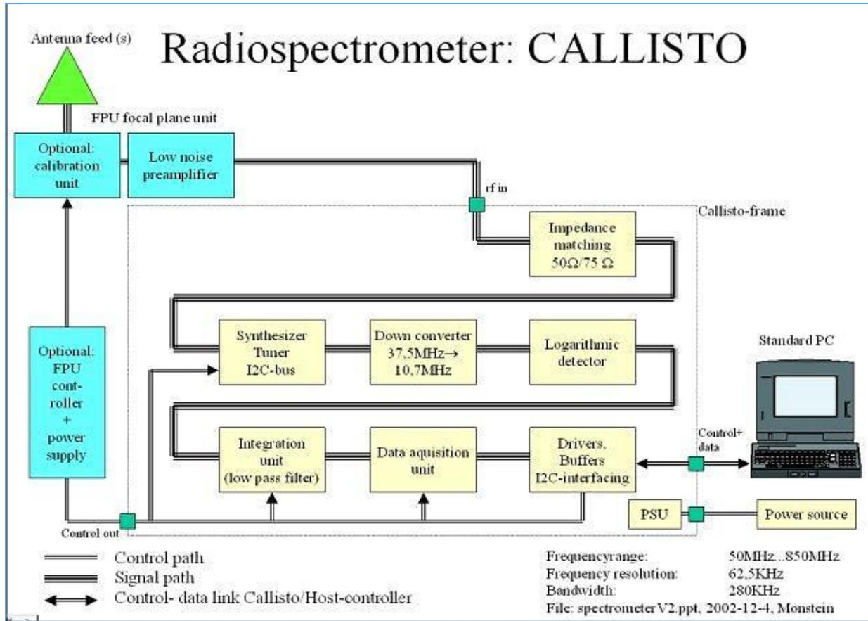
**Figure 2.** The flow of the process Radio Spectrometer CALLISTO (credited to e- CALLISTO)
