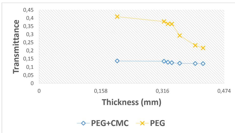
Fig. 2. The transmittance vs thicknesses for PEG and (PEG-CMC) films.
