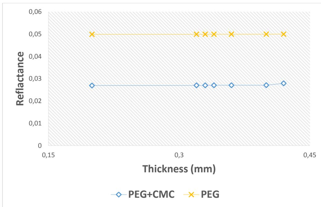
Fig. 3. Reflectance vs thicknesses for PEG and (PEG-CMC) films.
