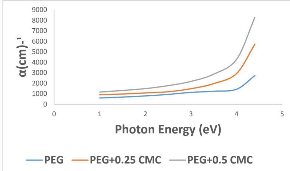
Fig. 4. Absorption coefficient vs photon energy for PEG and (PEG-CMC) films.
