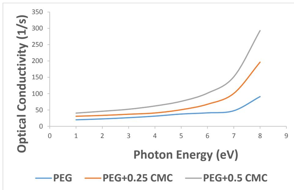
Fig. 10. Optical conductivity vs photon energy for PEG and (PEG-CMC) films.
