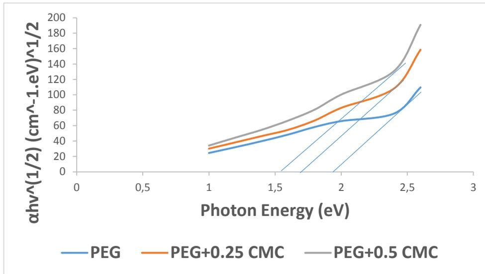
Fig. 5. Absorption coefficient vs photon energy for PEG and (PEG-CMC) films.
