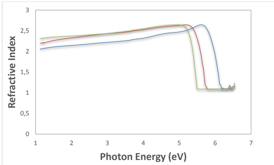
Fig. 6. Refractive vs photon energy for PEG and (PEG-CMC) films.
