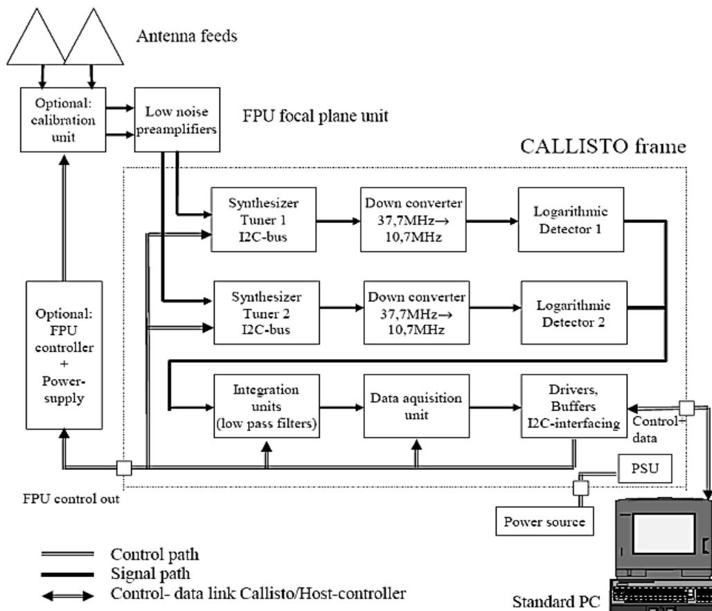
**Figure 3.** The basic design of the CALLISTO spectrometer with two receivers (top and middle row) operates in phase.
