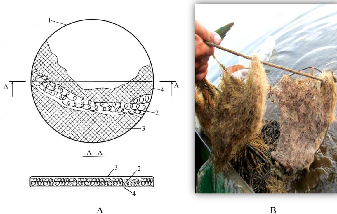
**Figure 8.** Artificial spawning nest: A – scheme of spawning nest: spawning nest, a top view and a sectional view along A-A: 1 – a metal frame 2 – spawning substrate 3–4 – upper and lower layers of the network fabric; B – general view of the established spawning nest
