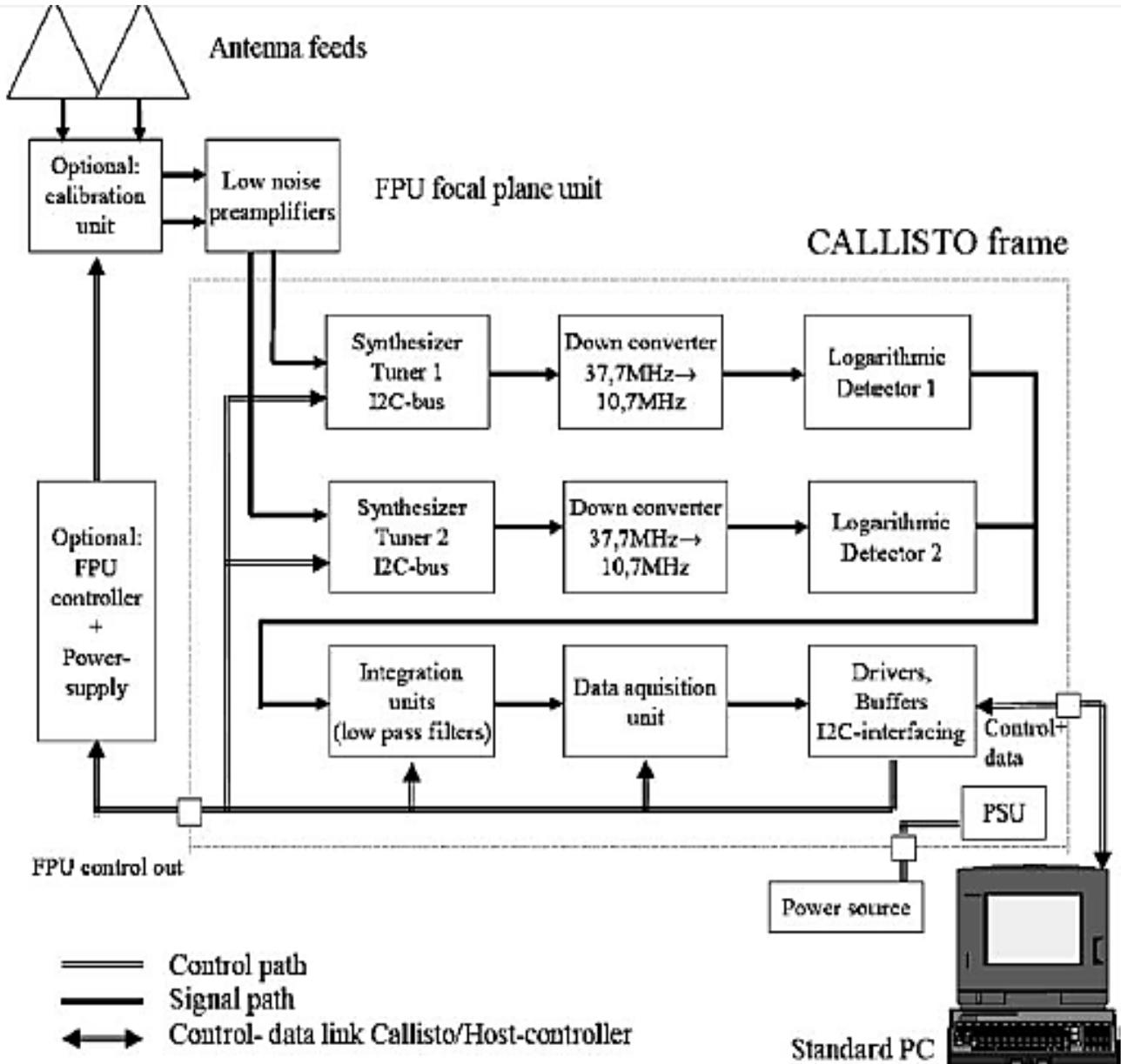
Figure 1. Basic design of solar radio spectrometer in radio observation
