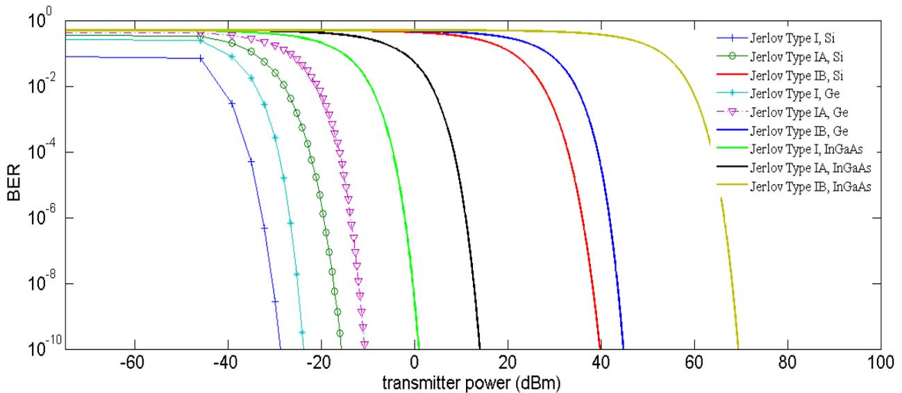
Fig. 9. BER versus transmitter power (dBm) when  $\theta = 1^\circ$ ,  $R = 100 \Omega$  and  $d = 35\text{m}$
