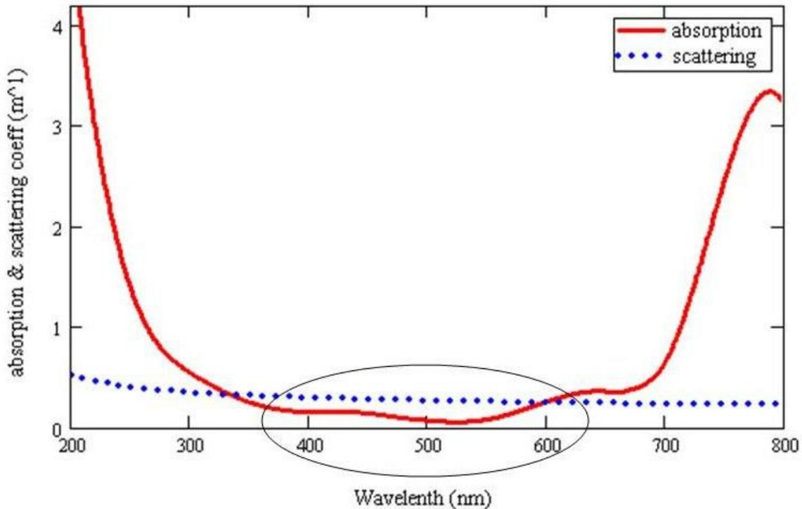
**Fig. 1.** Absorption and scattering coefficients of water with 1 mg/m<sup>3</sup> of chlorophyll concentration.
