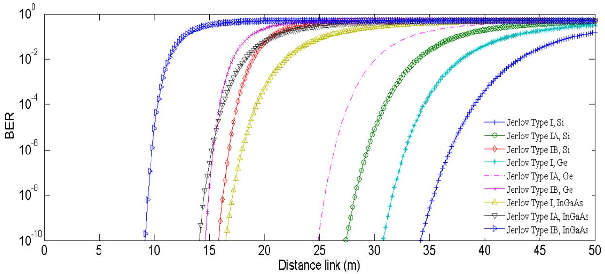
**Fig. 6.** BER versus distance link (m) when  $\theta = 1^\circ$ ,  $R = 100 \Omega$  and  $P_t = 50 \text{ mw}$
