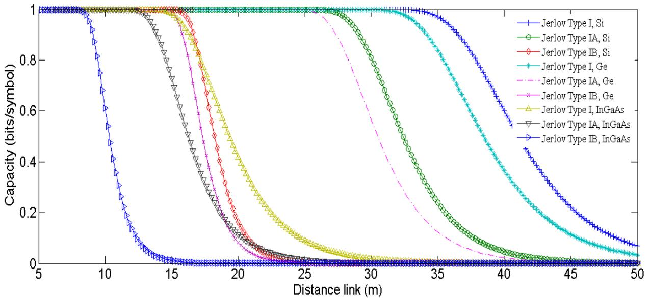
**Fig. 12.** Channel Capacity versus distance link (m) when  $\theta = 1^\circ$ ,  $R = 10 \Omega$  and  $P_t = 50 \text{ mw}$
