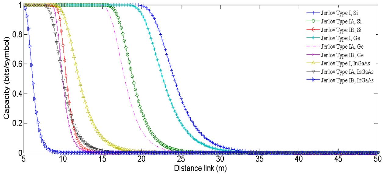
Fig. 13. Channel Capacity versus distance link (m) when  $\theta = 5^\circ$ ,  $R = 10 \Omega$  and  $P_t = 50 \text{ mw}$
