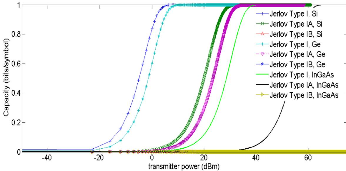
Fig. 15. Channel Capacity versus transmitter power (dBm) when  $\theta = 5^\circ$ ,  $R = 10 \Omega$  and  $d = 35 \text{ m}$
