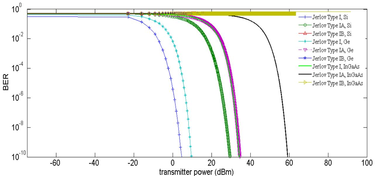
**Fig. 11.** BER versus transmitter power (dBm) when  $\theta = 5^\circ$ ,  $R = 100 \Omega$  and  $d = 35\text{m}$
