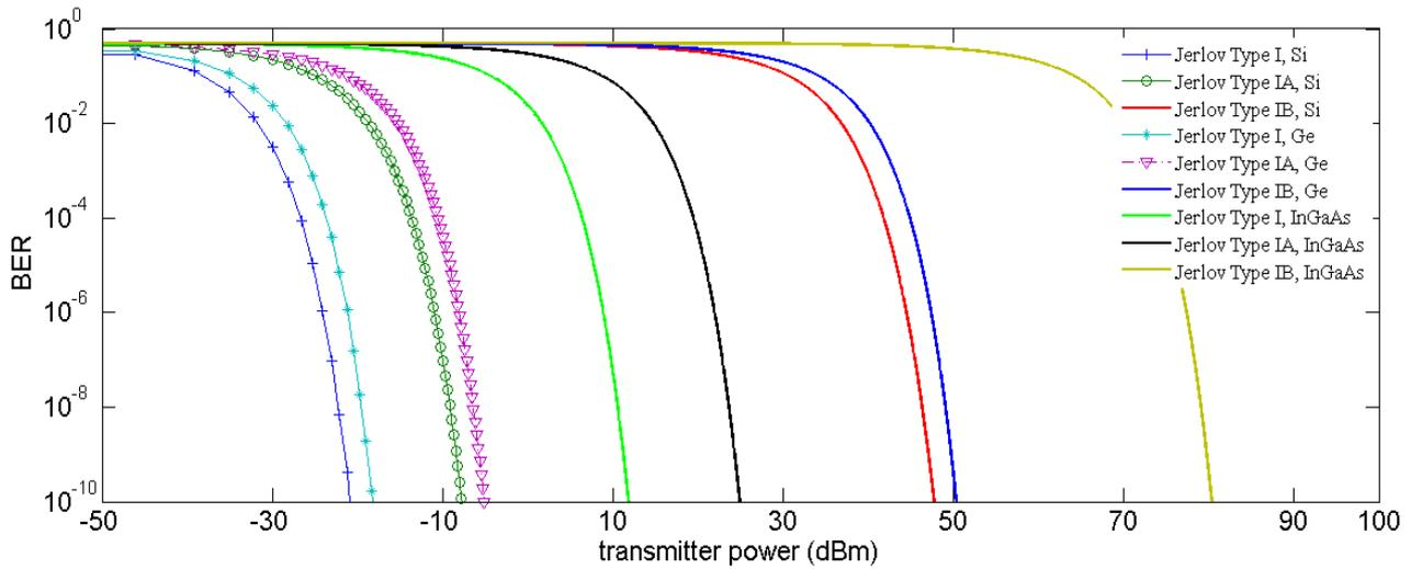
Fig. 8. BER versus transmitter power (dBm) when  $\theta = 1^\circ$ ,  $R = 10 \Omega$  and  $d = 35\text{m}$
