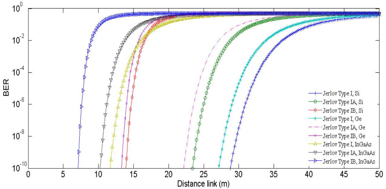
Fig. 4. BER versus distance link (m) when  $\theta = 1^\circ$ ,  $R = 10 \Omega$  and  $P_t = 50 \text{ mw}$
