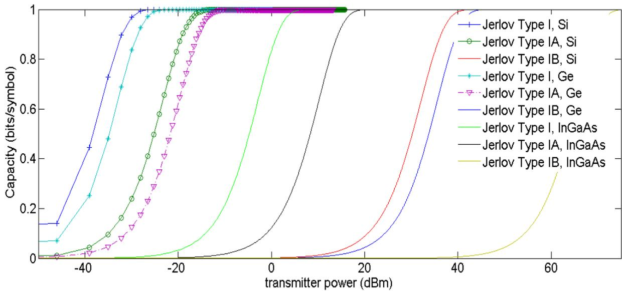
Fig. 14. Channel Capacity versus transmitter power (dBm) when  $\theta = 1^\circ$ ,  $R = 10 \Omega$  and  $d = 35 \text{ m}$
