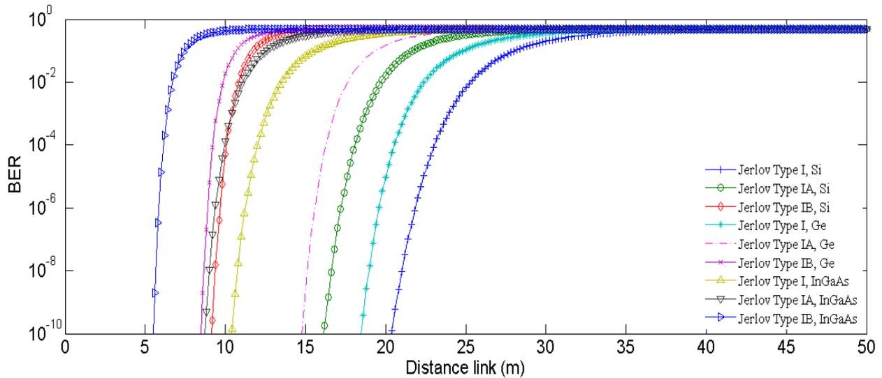
**Fig. 7.** BER versus distance link (m) when  $\theta = 5^\circ$ ,  $R = 100 \Omega$  and  $P_t = 50 \text{ mw}$
