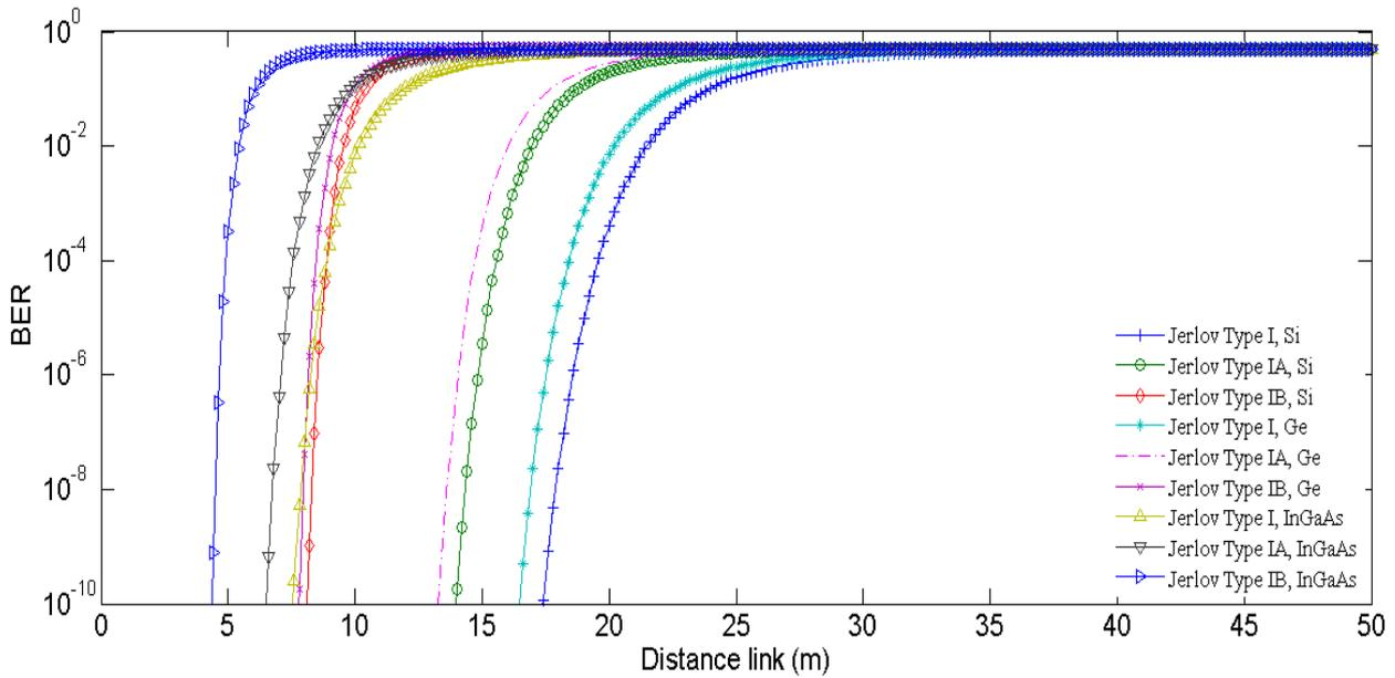
Fig. 5. BER versus distance link (m) when  $\theta = 5^\circ$ ,  $R = 10 \Omega$  and  $P_t = 50 \text{ mw}$
