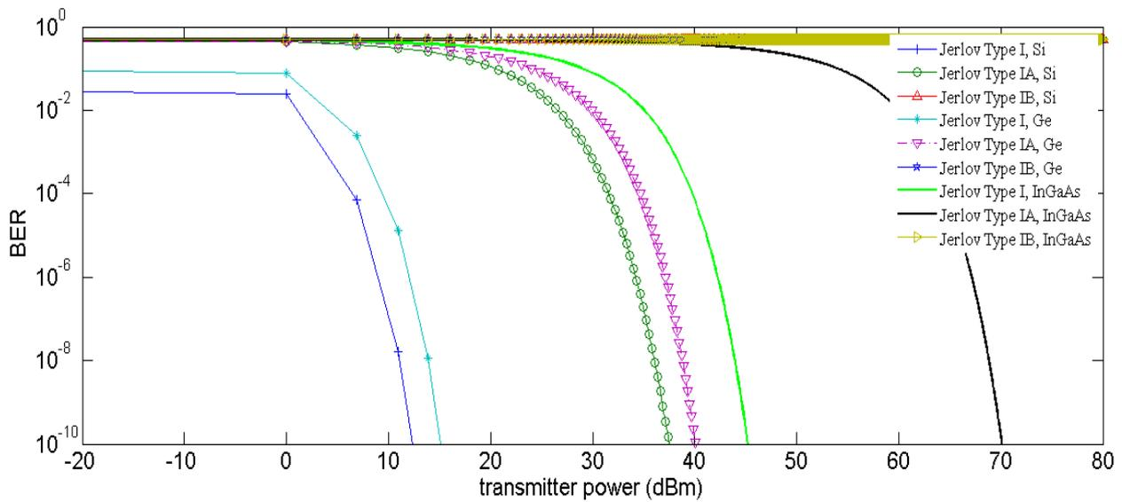
**Fig. 10.** BER versus transmitter power (dBm) when  $\theta = 5^\circ$ ,  $R = 10 \Omega$  and  $d = 35\text{m}$
