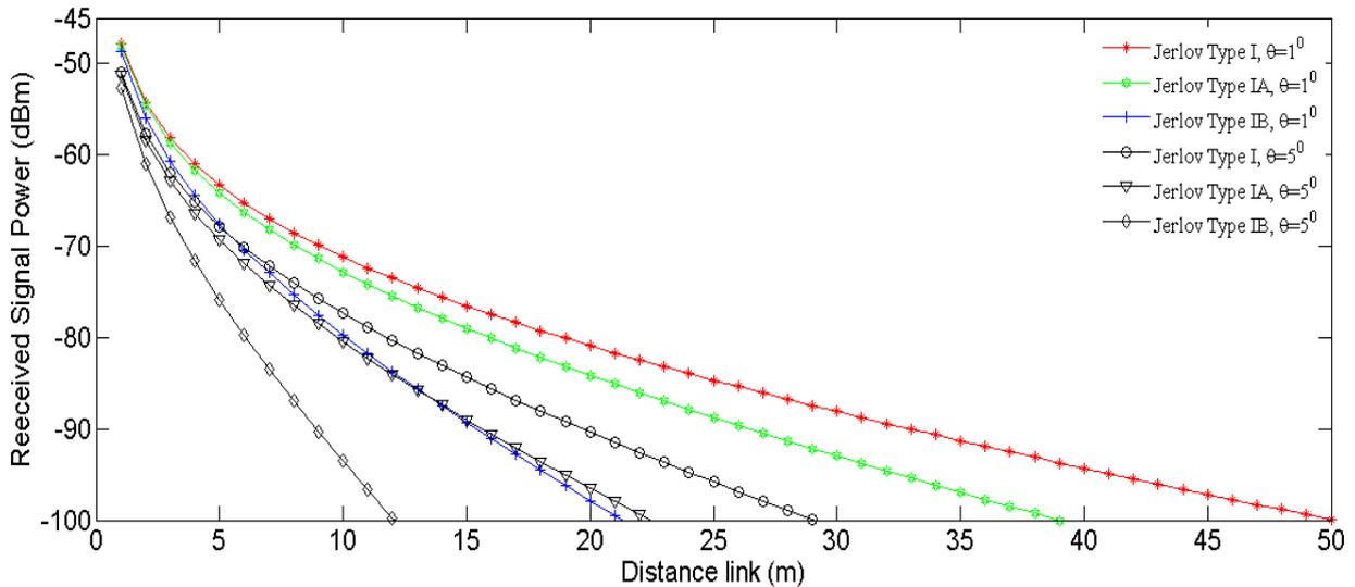
**Fig. 3.** Receiver signal power for an underwater environment
