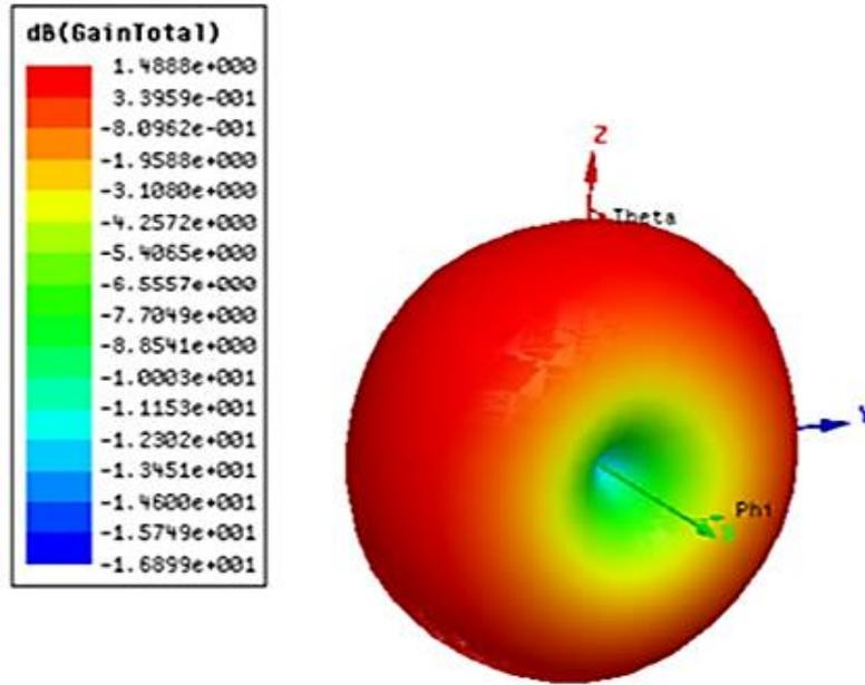
**Figure 8(b).** Magnitude vs. Frequency graphic and radiation pattern (Simulation).
