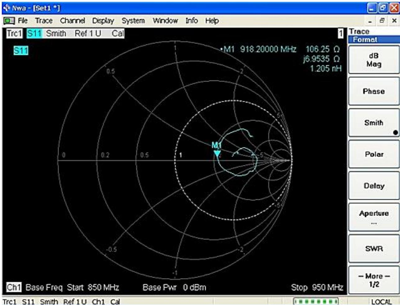
Figure 13. Antenna Impedance (Measurement).
