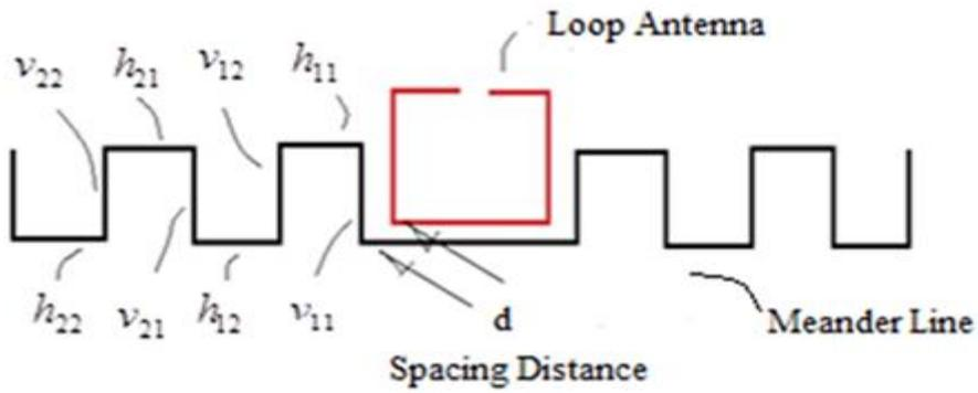
Figure 5(a). Uniform Meander Line Antenna.
