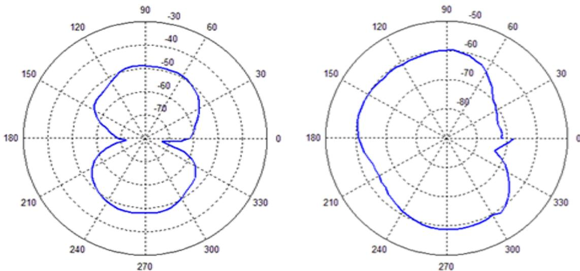
**Figure 10.** Magnitude vs. Frequency graphic and radiation pattern Plane E, Plane H (Measurement).
