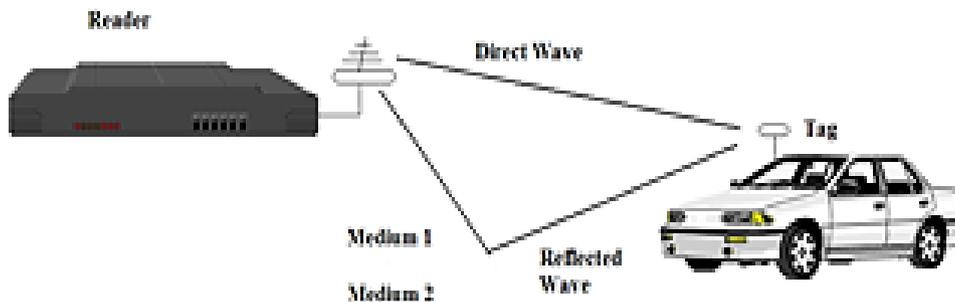
**Figure 3.** RFID technology applied to vehicular Identification.
