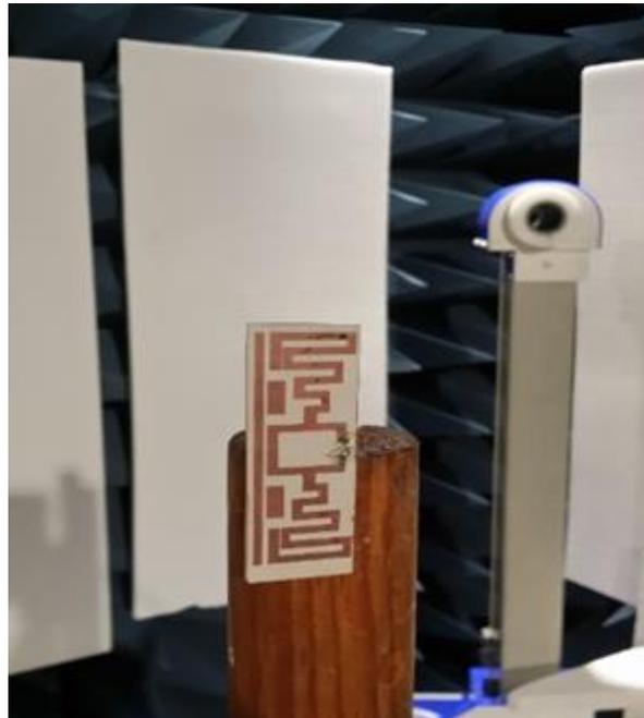
**Figure 9.** Prototype antenna under test (anechoic chamber).
