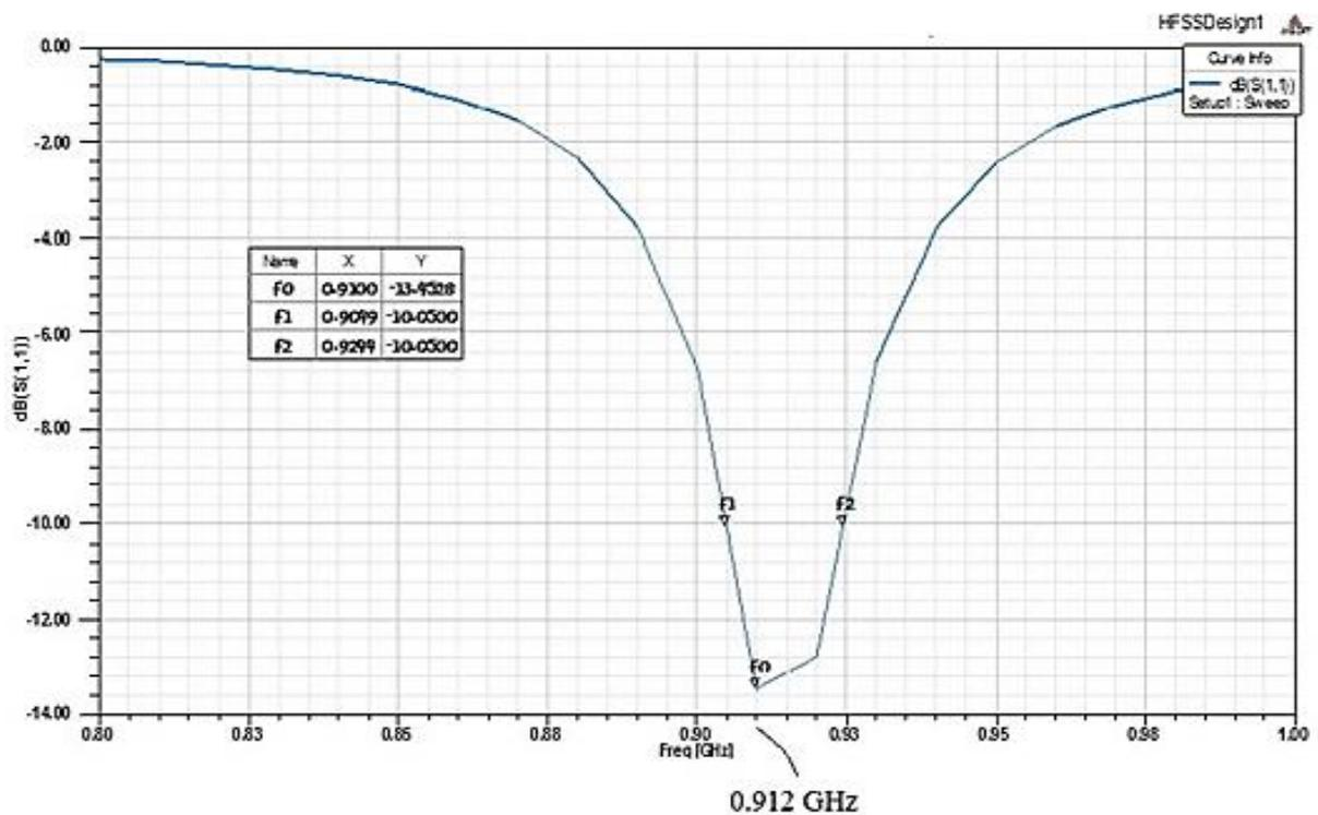
Figure 8(a). Magnitude vs. Frequency graphic and radiation pattern (Simulation).
