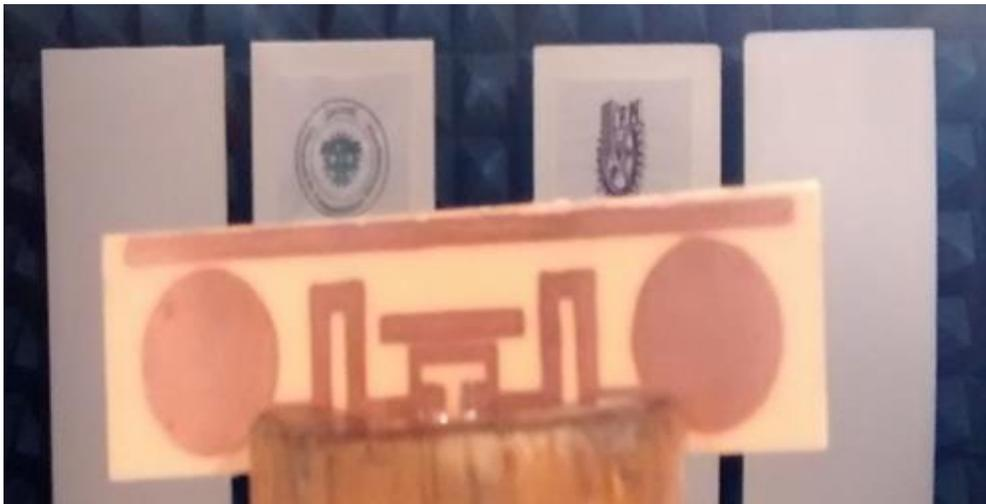
**Figure 11.** Prototype antenna under test (anechoic chamber).
