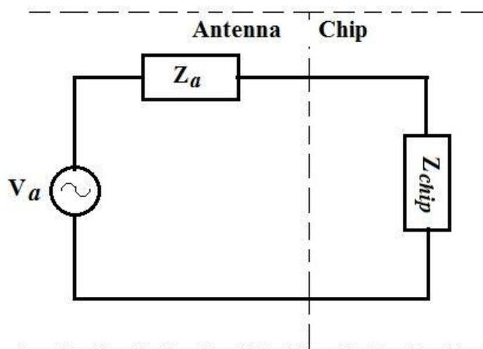
Figure 6(a). Inductive Match Feed Loop.
