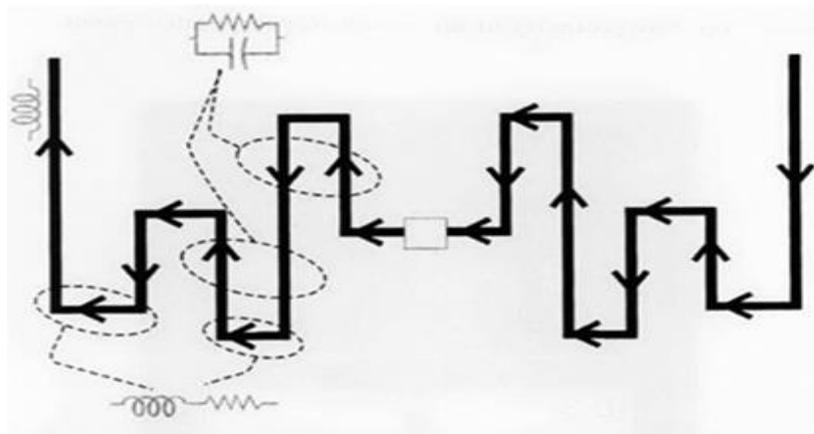
Figure 5(b). Uniform Meander Line Antenna.
