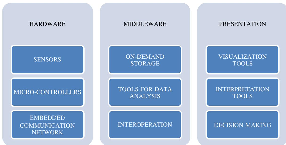
**Fig. 2.** Components of IoT
