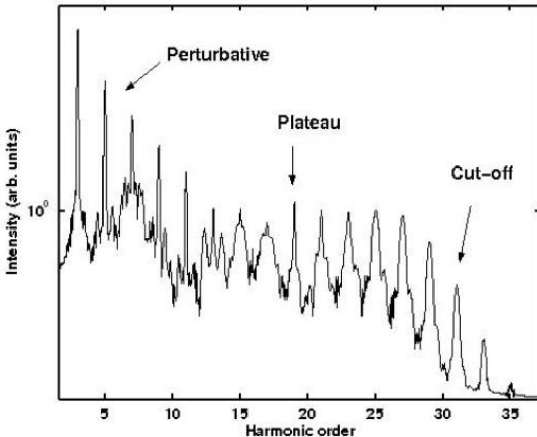
Figure 1. Harmonic spectrum of Argon using a laser peak intensity of  $1.4 \times 10^{18} \text{ Wm}^{-2}$  [2].
