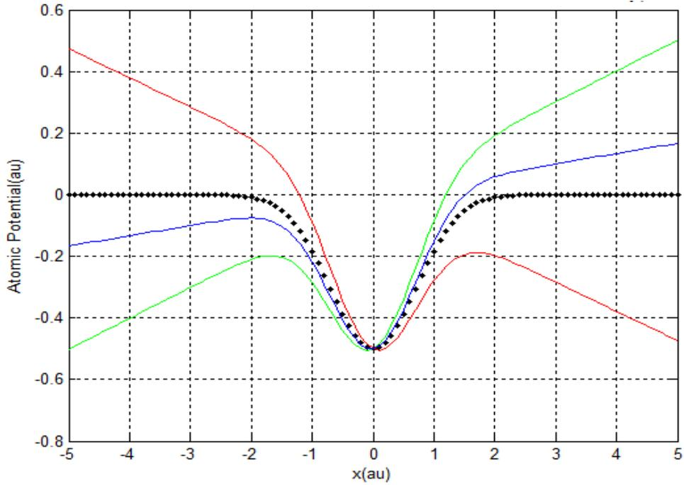
**Figure 4.** Atomic potential distortion due to cosine electric field intensity of  $5 \times 10^{18} \text{ Wm}^{-2}$ . Green red and blue, lines represent Ar, He-Ne and Ti-sapphire laser. Black lines are without an external laser field.
