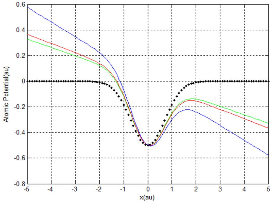
**Figure 8.** Atomic potential distortion due to sine electric field intensity of  $5 \times 10^{18} \text{ Wm}^{-2}$ . Green red and blue, lines represent Ar, He-Ne and Ti-sapphire laser. Black lines are without an external laser field.
