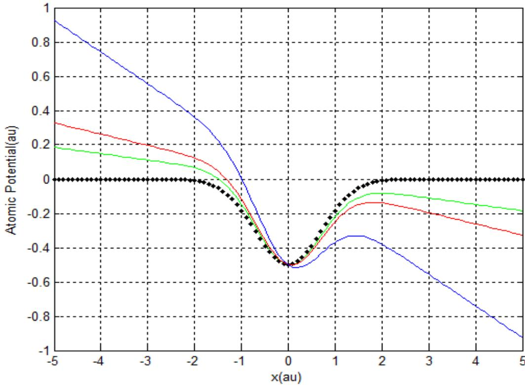
**Figure 7.** Atomic potential distortion due to the Ar laser field with different intensities (sine electric field) Blue, red and green lines represent intensity  $40 \times 10^{18} \text{ Wm}^{-2}$ ,  $5 \times 10^{18} \text{ Wm}^{-2}$  and  $1.6 \times 10^{18} \text{ Wm}^{-2}$ .
