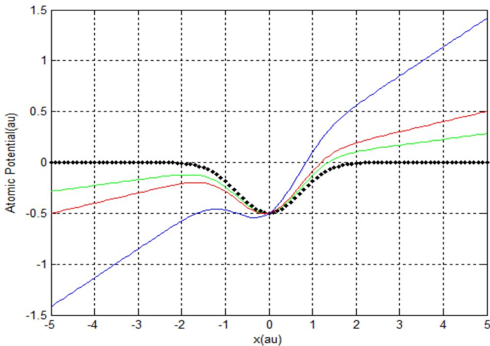
**Figure 3.** Atomic potential distortion due to the Ar laser field with different cosine electric field intensities. Blue, red and green lines represent the intensities,  $40 \times 10^{18} \text{ Wm}^{-2}$ ,  $5 \times 10^{18} \text{ Wm}^{-2}$  and  $1.6 \times 10^{18} \text{ Wm}^{-2}$ . Black lines are without an external laser field.
