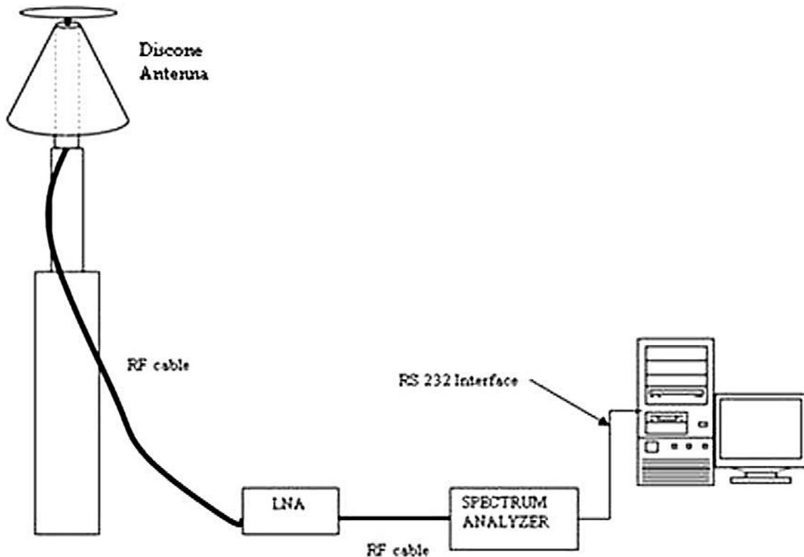
Figure 1. RFI system connection.
