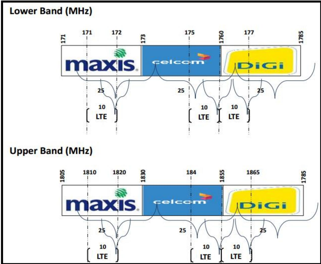
Figure 5. Global System for mobile 1800 (GSM1800) for Maxis, Celcom and Digi.
