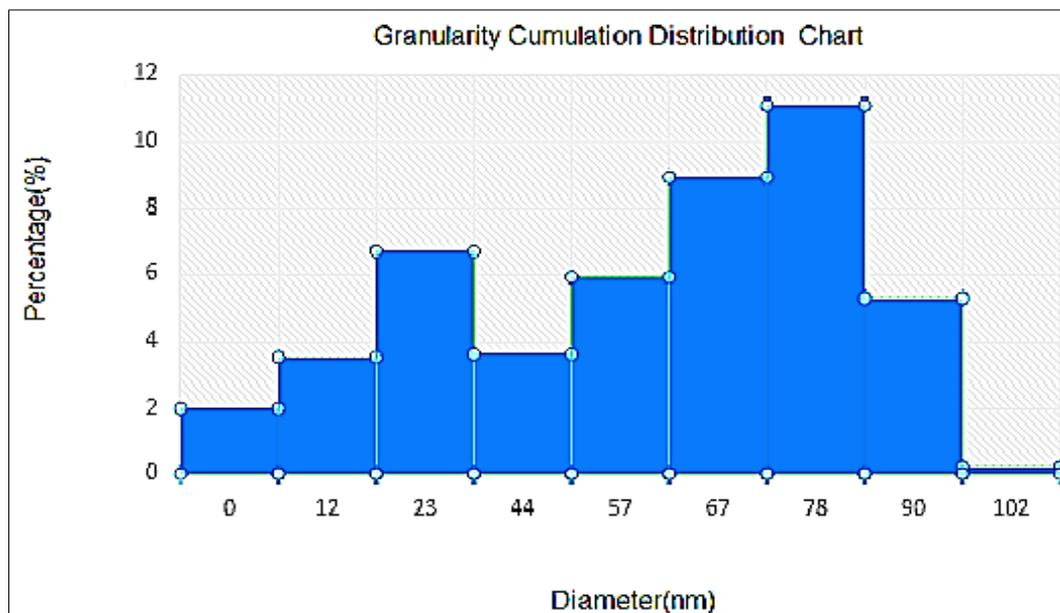
**Fig. 7.** Particle size distribution for copper nanocollid.
