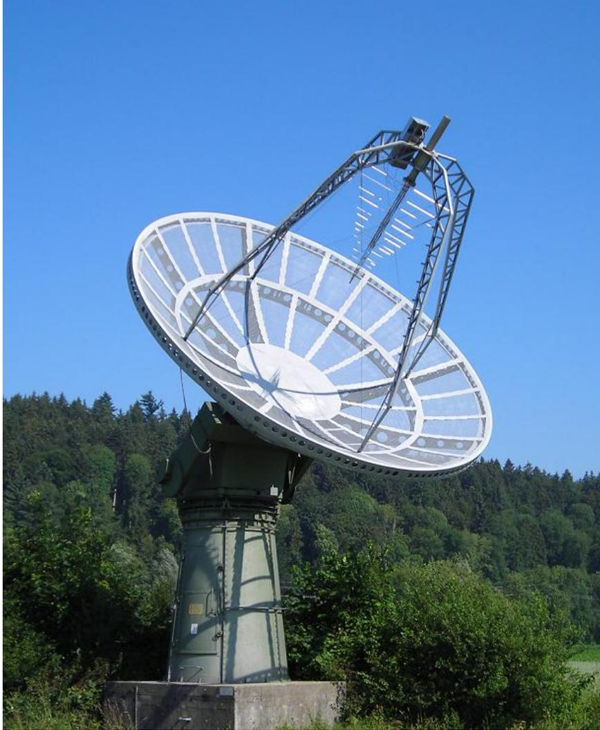
**Figure 2.** A 7 meter dish with a CALLISTO system at BLEIN site.
