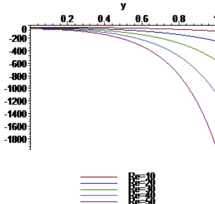
**Figure 2.** Velocity profile  $u$  against boundary layer  $y$  for varying Reynolds number  $Re$ .
