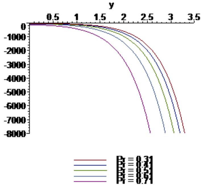
Figure 3. Velocity profile  $u$  against boundary layer  $y$  for varying Prandtl number  $Pr$
