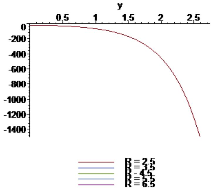
Figure 7. Velocity profile  $u$  against boundary layer  $y$  for varying Radiation  $R$
