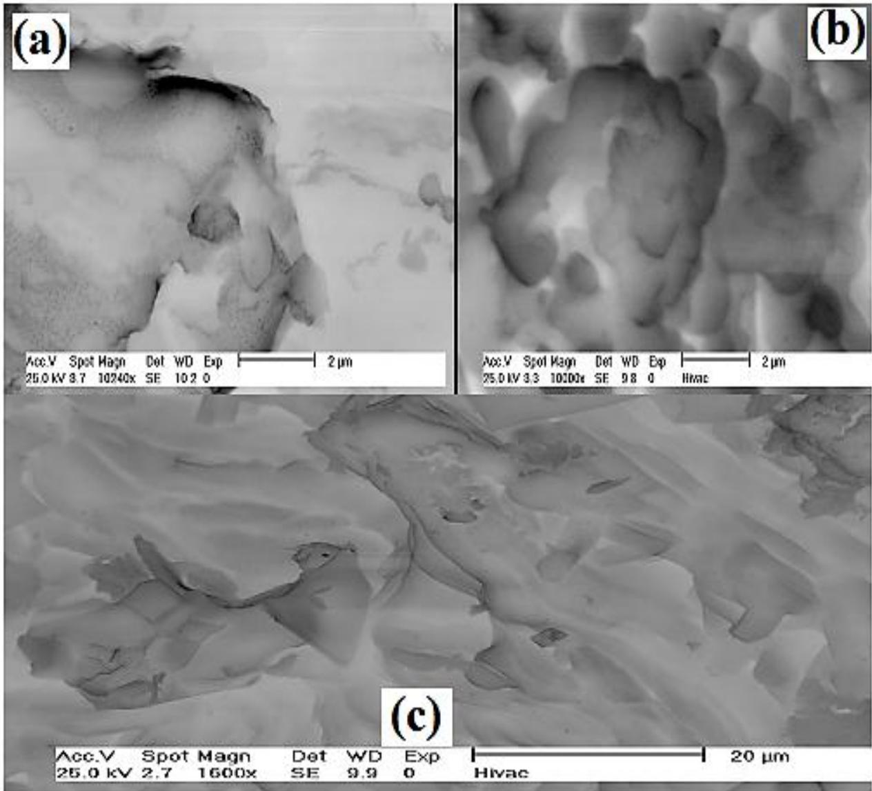
**Fig. 2(a-c).** SE-Micrographs recorded for In-doped – vanadates ceramics with general formula  $\text{Ca}_{3-x}\text{In}_x\text{VO}_8$ ; where; (a)  $x = 0.0$ , (b)  $x = 0.05$  and (c)  $x = 0.25$  mole, with different magnification factors 2 and 20  $\mu\text{m}$ .
