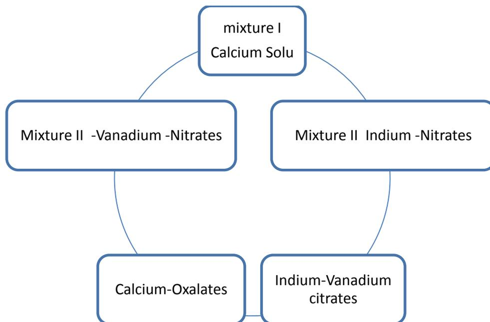
Schematic diagram show two different precursor applied for synthesizing Indium-doped vanadates.
