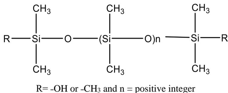
**Figure 1.** Chemical structure of the Polydimethylsiloxane (PDMS) polymer.
