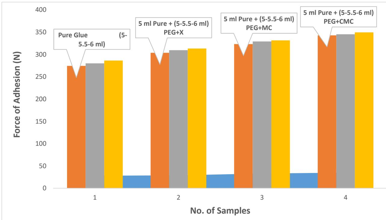
**Figure 9.** Adhesion Force for all samples.
