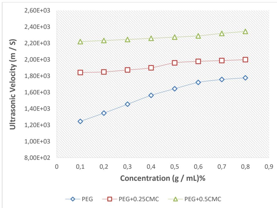
Figure 2. Ultrasonic velocity and concentrations.
