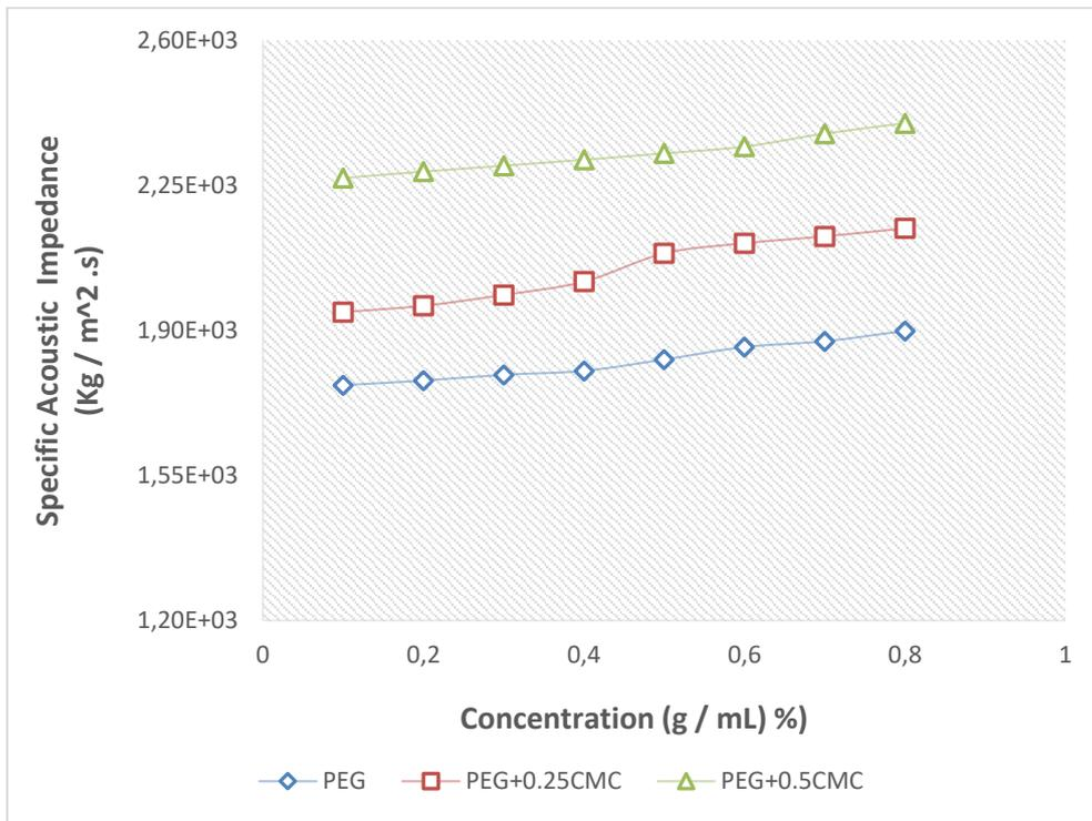
**Figure 7.** Specific acoustic impedance and concentration.
